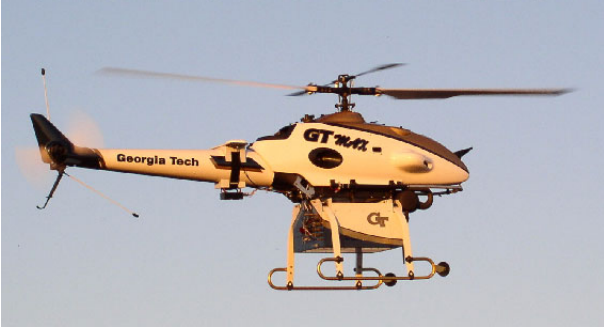
Fig. 8 GTMAX, autonomous helicopter test bed
