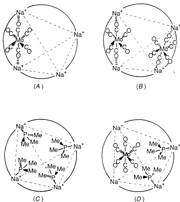
**Fig. 1** Summary of structural data for (A)  $8\{\text{Mo}(\text{CO})_6\}-\text{Na}_{56}\text{Y}$ , (B)  $16\{\text{Mo}(\text{CO})_6\}-\text{Na}_{56}\text{Y}$ , (C)  $32\{\text{PMe}_3\}-\text{Na}_{56}\text{Y}$  and (D)  $8\{\text{Mo}(\text{CO})_6\}, 16\{\text{PMe}_3\}-\text{Na}_{56}\text{Y}$
