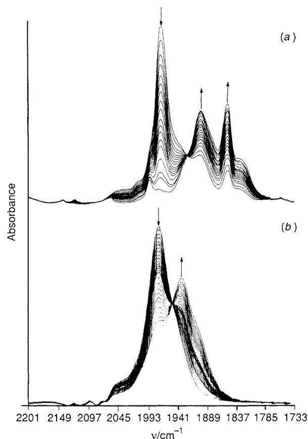
**Fig. 2** Typical mid IR spectral changes observed for (a)  $n\{\text{Mo}(\text{CO})_6\}, m\{\text{PMe}_3\}-\text{Na}_{56}\text{Y}$  and (b)  $n\{\text{Mo}(\text{CO})_6\}, m\{^{13}\text{CO}\}-\text{Na}_{56}\text{Y}$  [ $P(^{13}\text{CO}) = 100$  Torr],  $T = 65.8$  °C]
