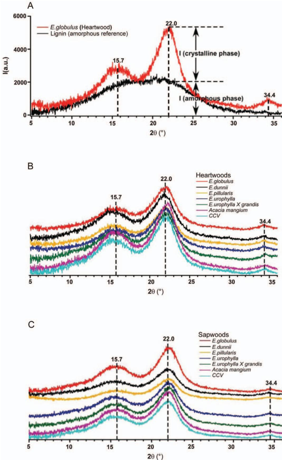
**Figure 2. X-ray diffractograms of heartwood and sapwood samples.** (A) Example of eucalyptus species (*E. globulus*) and reference (lignin) x-ray diffractogram to determine amorphous and crystalline phase. X-ray diffractograms of heartwoods (B) and sapwoods (C) of all hardwood species. doi:10.1371/journal.pone.0052820.g002
