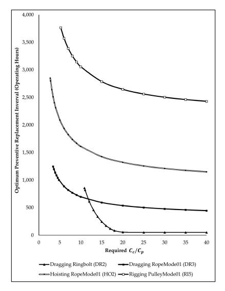
Figure A2. Optimal replacement intervals of Dragline-2 wear-out components for changing cost ratios.
