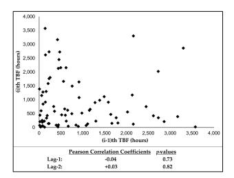
Figure 3. Data independency tests for lifetime dataset of Dragline-1 bucket pin.
