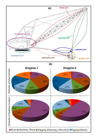
Figure 2. Decomposition of dragline (a) and distribution of maintenance statistics (b).
