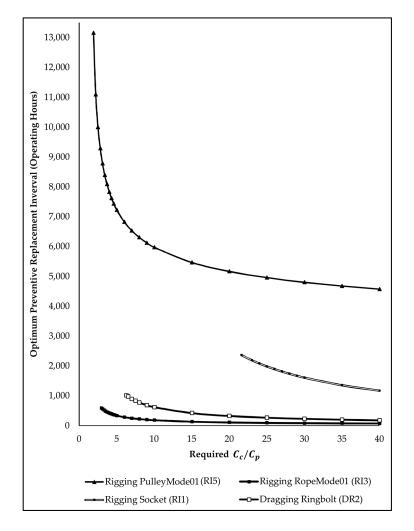
Figure A1. Optimal replacement intervals of Dragline-1 wear-out components for changing cost ratios.
