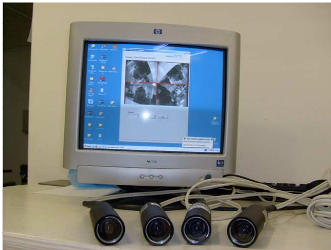
Figure 7.5: 4 pieces of BWC-300 underwater cameras and synchronous video capturing with these cameras.
