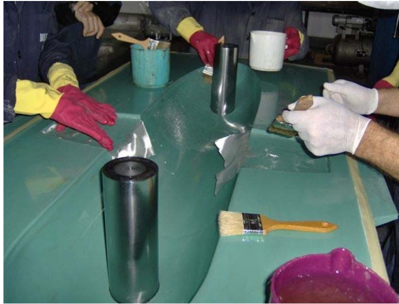
Figure 6.4 Hand lay-up process for the vehicle body
