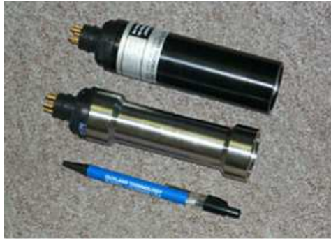
Figure 7.2: Outland Tech. UWC-300 underwater cameras (black cylinder, top)
