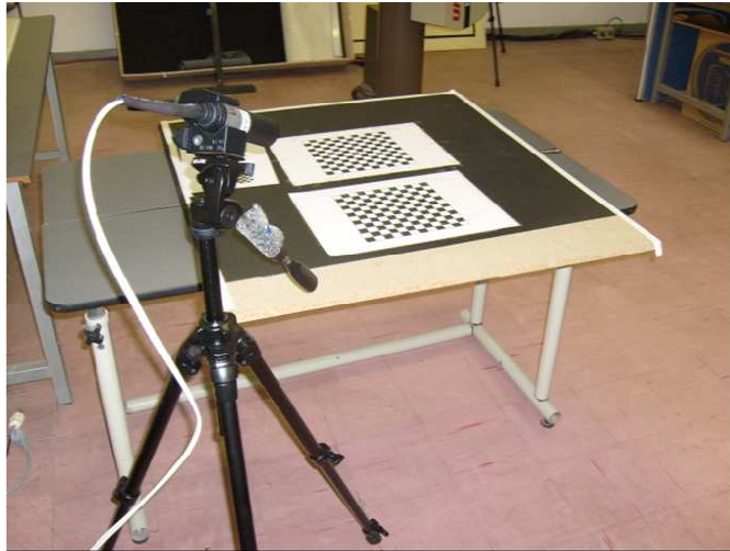
Figure 7.4: Tripod-clamp-camera trio and the calibration pattern. (Shown for a single camera)
