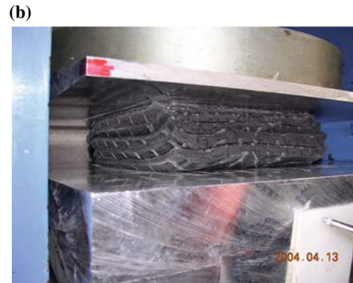
Fig. 7 Inclined compression test setup
