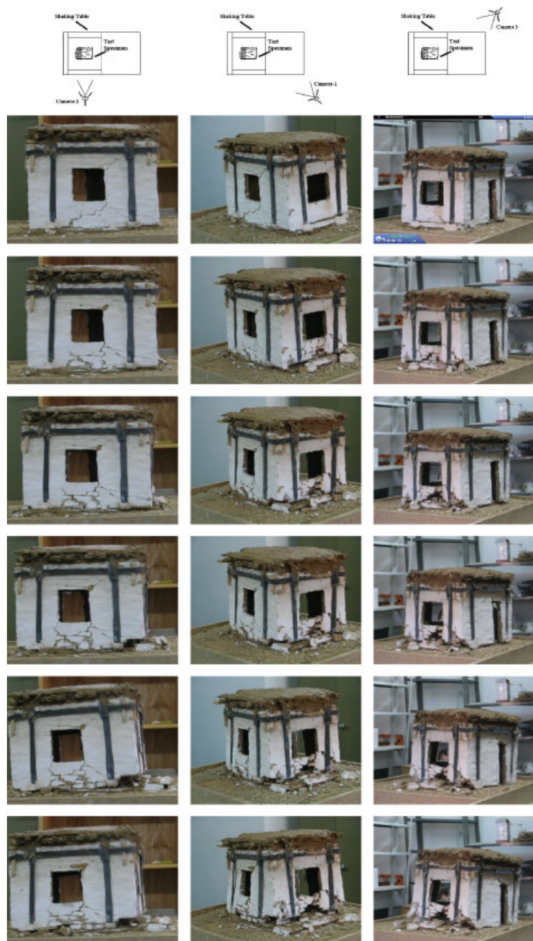
Figure 16. Failure sequence of specimen (VHSS2).
