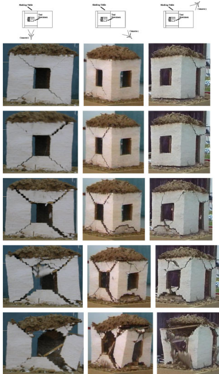
Figure 11. Failure sequence of specimen (RFO2).
