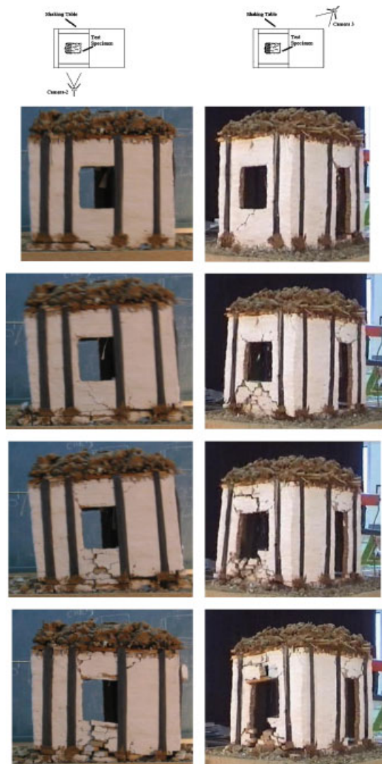
Figure 14. Failure sequence of specimen (VSS).
