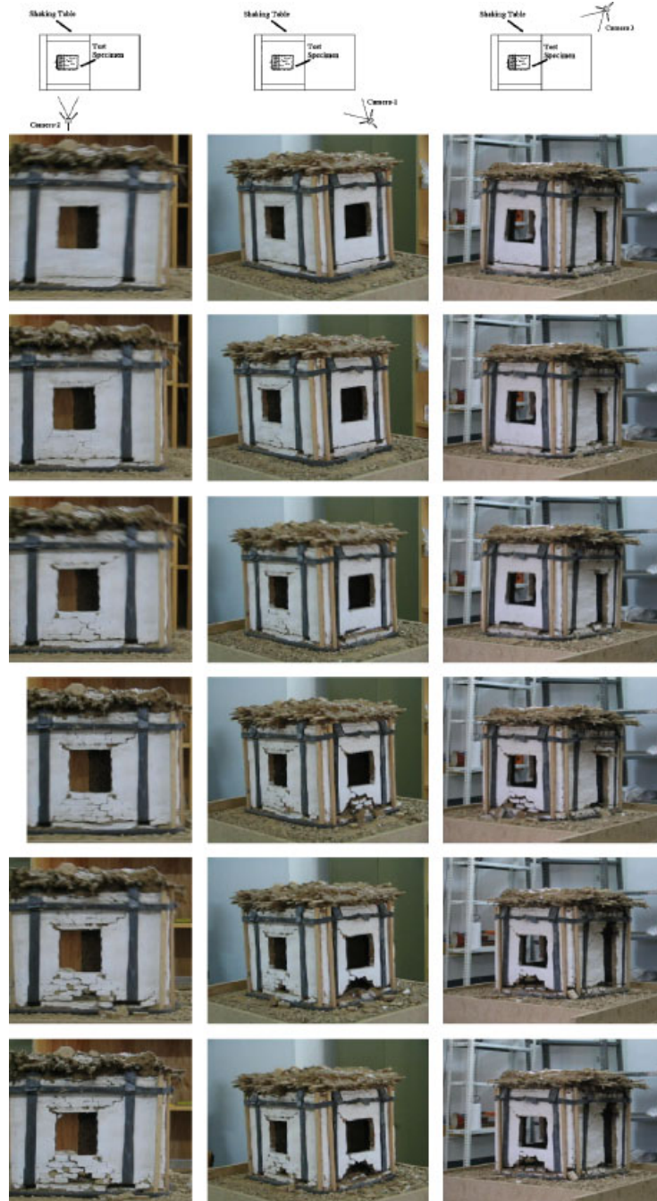
Figure 15. Failure sequence of specimen (VHSS1).
