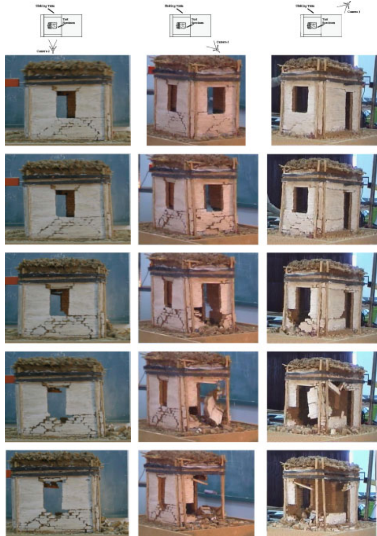
Figure 12. Failure sequence of specimen (HSS1).
