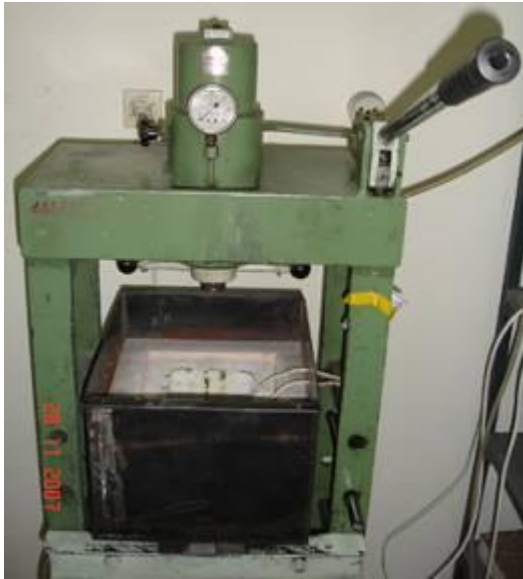
Figure 2 The system used in production (a) hot press and (b) die
