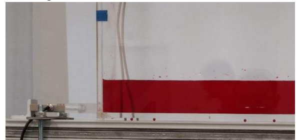
Figure 12. Load cell assembly
