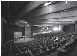
**Figure 4.** Learning Laboratory: Radial Reinforced concrete beams, waffle slabs.
