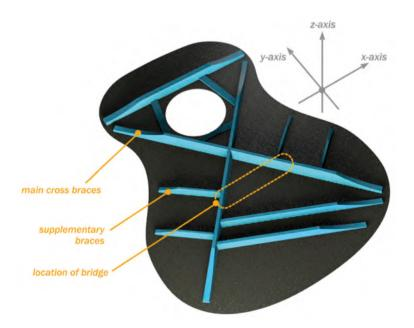
**Figure 1.** Underside of generic X-braced soundboard showing x-, y- and z-axis stresses.
