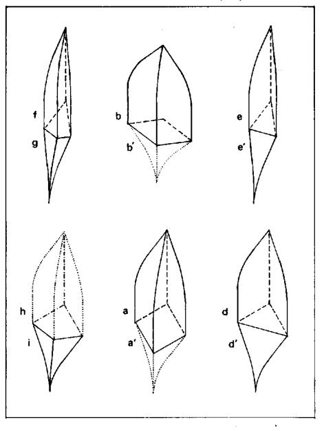
Figure 4. Three dimensional elements of the arched stalactite.
