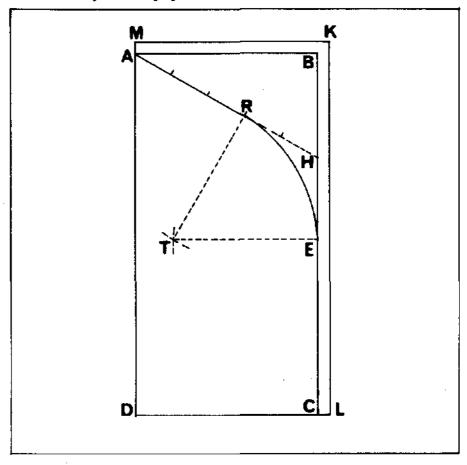
Figure 5. Pattern drawing for the arched and Shirazi stalactites, (illustrated by el-Kashi). 25. El-Kashi makes a calculation error. The correct value should be 0,960770. This error repeats itself in the following calculations wherever EC is invoved.
