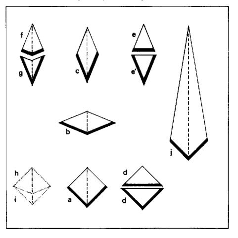
Figure 3. Ceiling elements of the simple stalactite (illustrated by el-Kashi).
