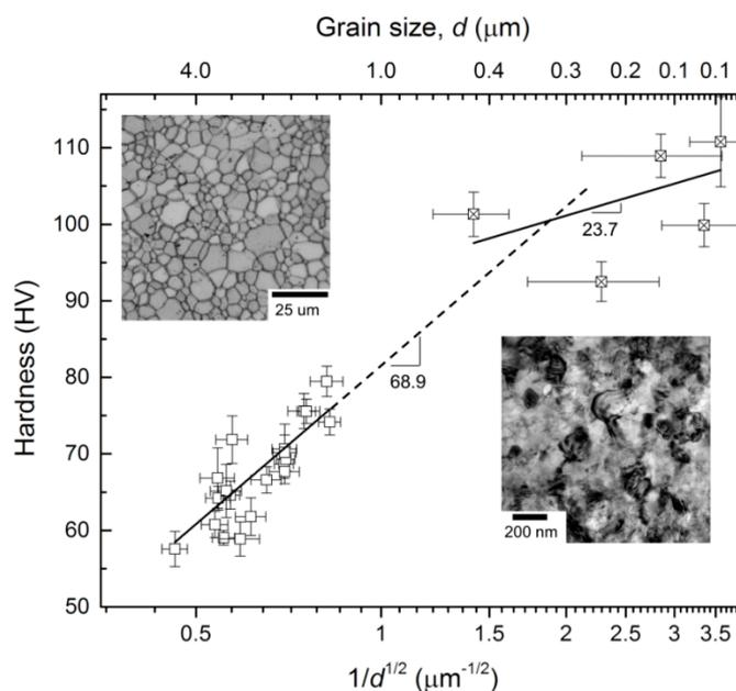
**Figure 7.** Hall-Petch plot showing the slope change in the sub-micron grain size regime. Characteristic microstructures corresponding to fine-grained and UFG regimes are shown.
