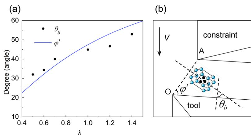
**Figure 4.** Strain path effect on texture in LSEM: (a) dependence of B-fiber orientation on  $\lambda$ ; solid curve shows the  $\varphi'$  variation with  $\lambda$ ; (b) schematic showing the alignment of basal plane parallel to the shear plane.
