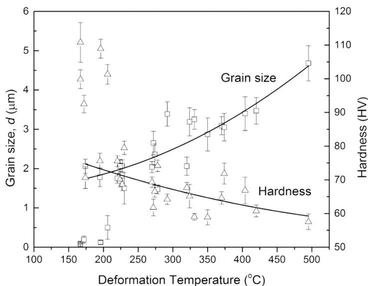
**Figure 5.** Variation of grain size ( $d$ ) and hardness with deformation temperature,  $T$ . Lines (polynomial fit) drawn to guide the eye.
