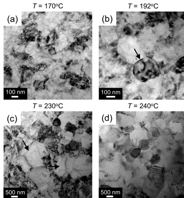
**Figure 6.** Bright-field TEM images showing the microstructural transitions with  $T$ . Note the different magnifications of the images.
