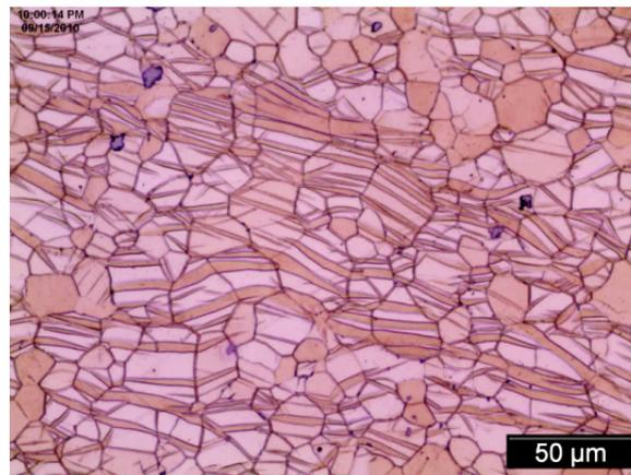
**Figure 2.** Subsurface twinned layer in the workpiece;  $\lambda = 1$ ,  $t = 250$   $\mu\text{m}$ ,  $V = 1$  m/s and  $T_o = 25^\circ\text{C}$ .
