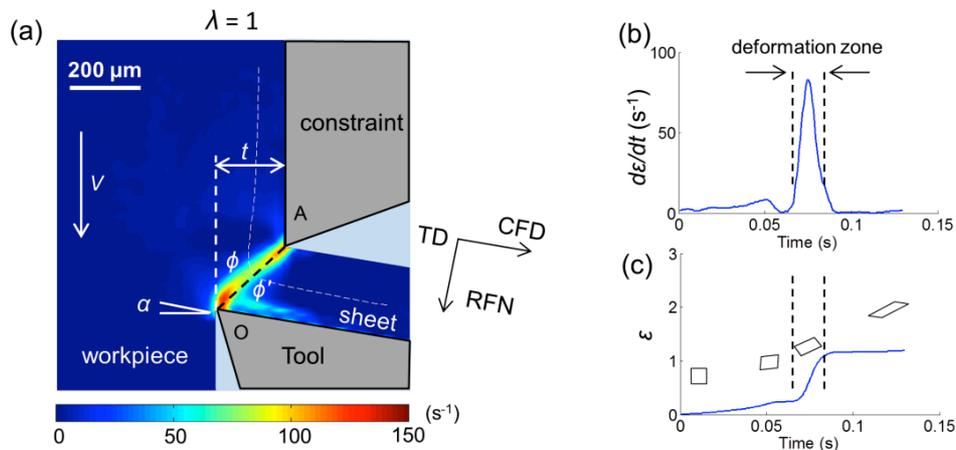
**Figure 1.** Deformation in LSEM: (a) strain-rate field showing the confined deformation zone; strain-rate (b) and accumulated strain (c) profiles along a pathline across the deformation zone. CFD is the chip flow direction, RFN the rake face normal and TD the transverse direction. Workpiece is commercially pure lead,  $\lambda = 1$ ,  $t = 200 \mu\text{m}$ ,  $\alpha = 10^\circ$  and  $V = 10 \text{ mm/s}$ .
