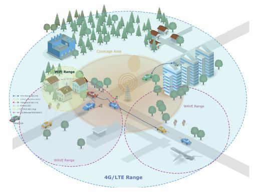
Figure 1. Heterogeneous vehicular networks in IoV.
