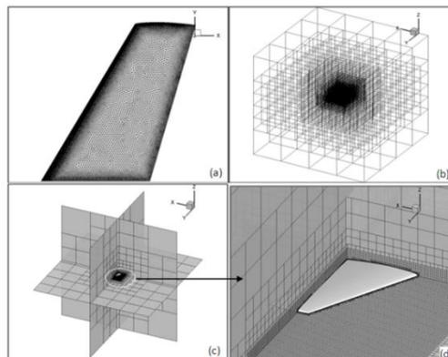
Fig. 8. (a) Magnified outlook of the surface grid of the ONERA M6 wing on XY plane, (b) isometric view of the Cartesian grid solution domain around the wing, (c) sliced expression of the whole domain wing-centred, (d) close-up view on the grid.
