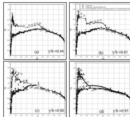
Fig. 10. GeULER-NaTure viscous, turbulent flow results of pressure coefficient ( $c_p$ ) distributions versus  $x/c$  on the surface of transonic ONERA M6 wing test case at (a)  $y/b=0.44$ , (b)  $y/b=0.65$ , (c)  $y/b=0.80$ , (d)  $y/b=0.95$ ;  $M_\infty=0.8395$ ,  $\theta = 3.06^\circ$ ,  $Re = 11.7 \times 10^6$ .
