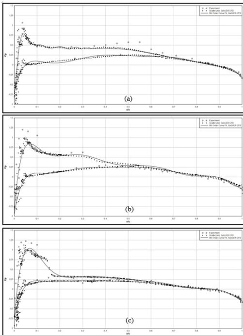
**Fig. 11. GeULER-NaTURE inviscid, laminar flow results of pressure coefficient ( $C_p$ ) distributions versus  $x/c$  on the surface of transonic ONERA M6 wing test case at (a)  $y/b=0.44$ , (b)  $y/b=0.80$ , (c)  $y/b=0.95$ ;  $M_\infty=0.8395$  and  $\theta = 3.06^\circ$  (Kara *et al.*, 2016).**
