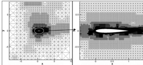
**Fig. 2. Mesh generation after three level solution adaptation around NACA 0012.**
