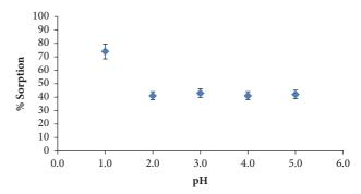
FIGURE 1: Effect of pH on sorption. Amount of resin: 0.1 g resin, amount of DEBT: 1mmol g<sup>-1</sup> resin, and stirring time: 50 minutes.
