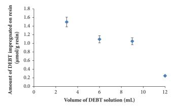
FIGURE 4: Effect of ligand volume on impregnation. Initial DEBT-ethanol concentration:  $3.75 \times 10^{-4} \text{ mol L}^{-1}$  and flow rate:  $0.5 \text{ mL min}^{-1}$ .
