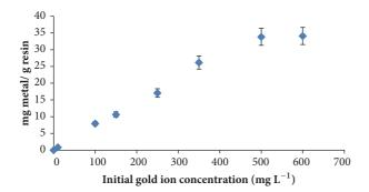
Figure 3: Gold ion capacity of resin. Amount of resin: 0.1 g, amount of DEBT: 1 mmol g $^{-1}$  resin, and stirring time: 15 minutes.
