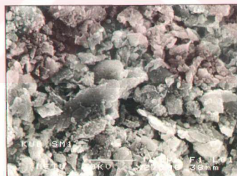
Figure 3.44 A close SEM view of the mortar matrix of Kubadabad Palace (kub.SM1) x 2000
