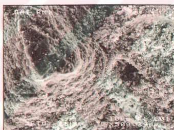
Figure 3.48 SEM view showing the good adhesion between a coarse aggregate and the mortar matrix of the minaret of Hatuniye Mescidi (hat.BM1) x 500
