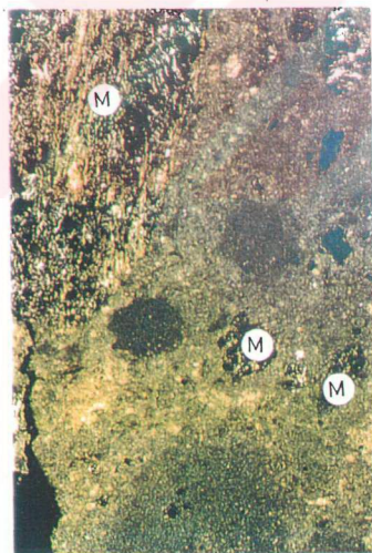
Figure 3.26 Metamorphic rock fragments in Taşmedrese mortar (teşe.SM1) M: metamorphic rock fragment
