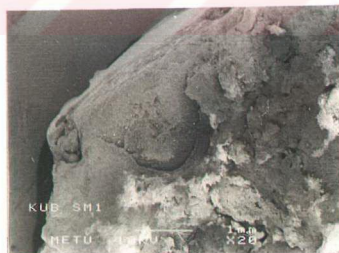
Figure 3.54 SEM view of the C-S-H formation in the mortar matrix of Kubadabad Palace (kub.SM1) x 20
