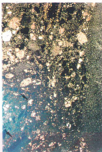
Figure 3.25 Abundant presence of biotite in the mortar of Zenburi Mescidi (zen.BM1)
