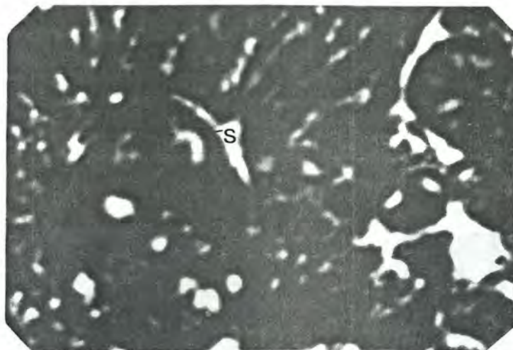
Figure 30. Selliporella grainstone. Selliporella donzellii (s) in sparitic groundmass. A.1518-1520 m , x 40 Burhandere formation.
