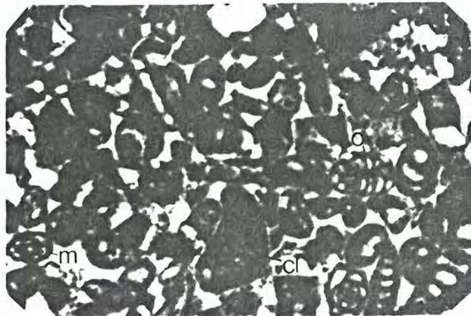
Figure 13. Miliolid grainstone. Miliolids (m), clasts (cl), Orbitolinopsis (o) in sparitic groundmass. A.260-262 m, x 40. Burhandere formation.
