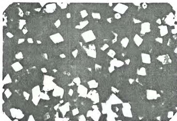
Figure 15. Dolomitized mudstone. Well crystallized dolomite rhombs in pure lime mud. A.390-392 m., x 40. Burhandere formation.
