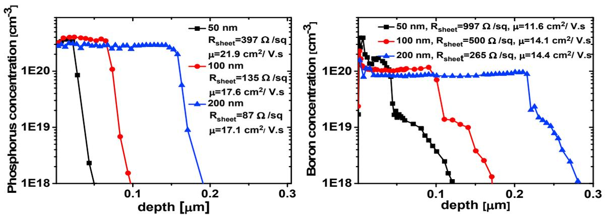
Fig.2. Doping profiles for the phosphorus (a) and boron (b) doped polySi/SiO<sub>x</sub>/Cz-Si carrier selective contact layers with their corresponding  $R_{sheet}$  values, on polished wafers. The nominal thickness of the polySi layers before the doping was 50 nm, 100 nm and 200 nm.
