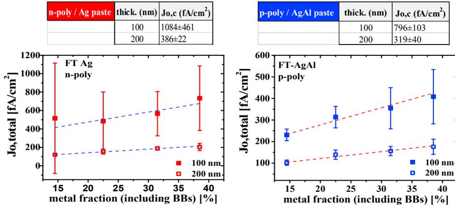
Fig. 6.  $J_{o,total}$  vs. metal fraction, and extracted  $J_{o,c}$  values for nominally 100 and 200nm thick n-polySi, metallized with FT-Ag paste (left) and p-polySi metallized with FT-Ag/Al paste (right). Samples were fired with a set peak temperature of 825°C. The error margins are the standard deviation of the measurement of multiple cells with the same metal coverage on one wafer.
