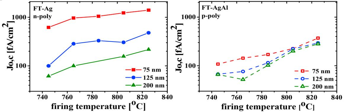
Fig. 5. Modelled  $J_{o,c}$  for FT Ag paste on n-poly/wafer/n-poly (left) and FT AgAl paste on p-poly/wafer/p-poly (right) for 75, 125 and 200 nm poly layers fired at five different firing temperatures.
