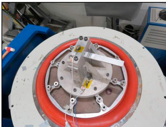
Fig. 6 The vibration fatigue test setup of the notched beams
