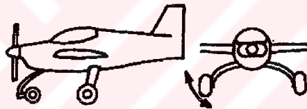
Figure 9.6 Solid spring type of gear/shock arrangement. [1]
