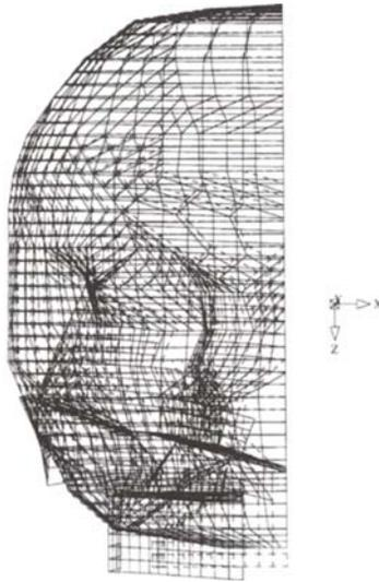
**Figure 3** Pattern of computed displacements (----- unloaded; ——— loaded) of the nasomaxillary complex, with 5 mm of RME. Note that the centre of rotation is located at the frontal bone.
