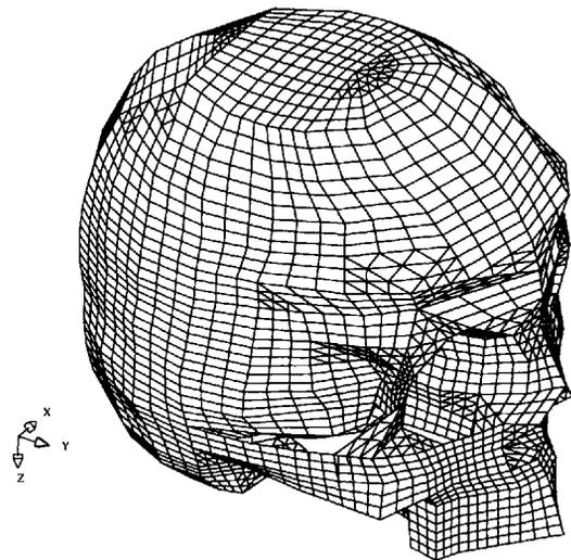
**Figure 2** Three-dimensional finite element model of the craniofacial complex. The model consists of 2349 quadrilateral and triangular thick shell elements with 2147 nodes. At each node three translational and three rotational degrees of freedom are defined.
