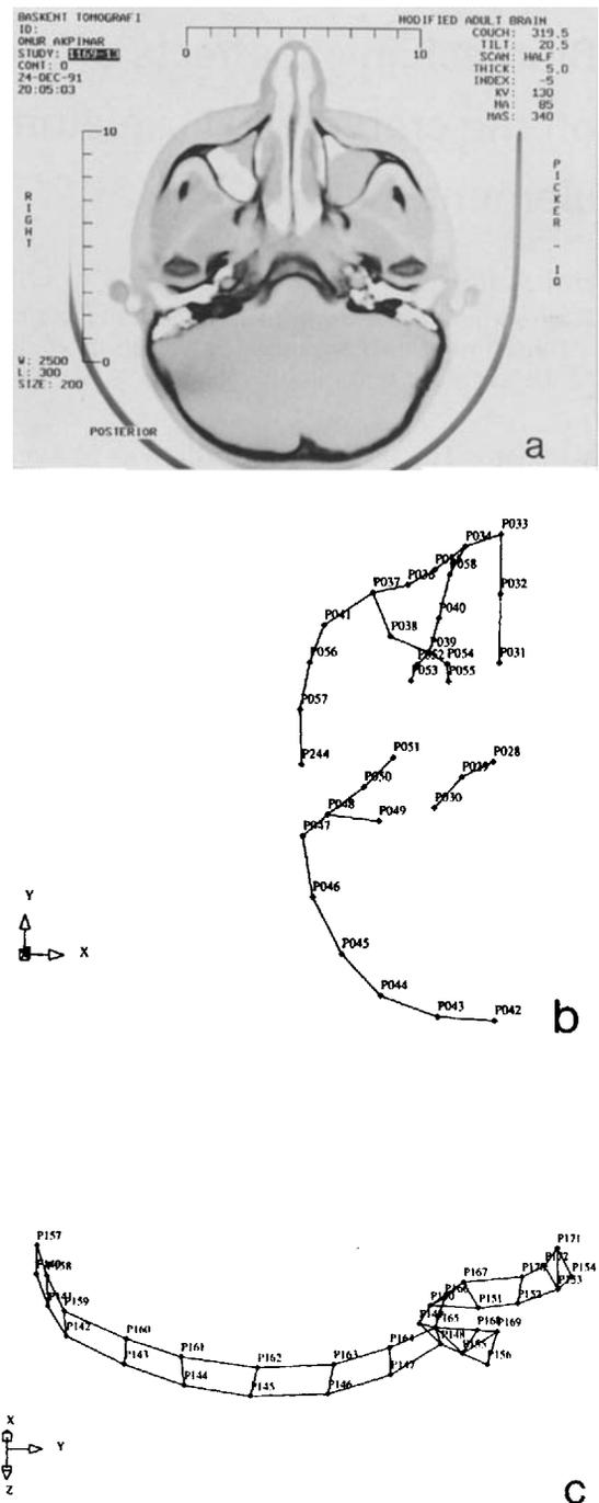
**Figure 1** Basic steps of generating the finite element model of the cranium: (a) Sample slices obtained by computer tomography. (b) Geometric lines generated by using geometric points assigned along the midline of the skull bone. (c) Geometric surfaces generated from geometric lines.
