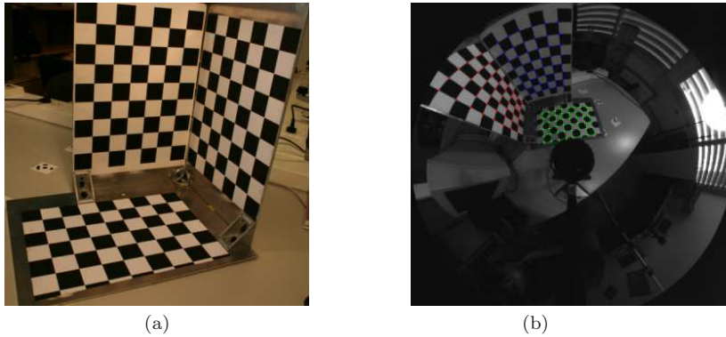
Fig. 5 (a) 3D pattern, (b) Omnidirectional image of the 3D pattern (1024×768 pixels).
