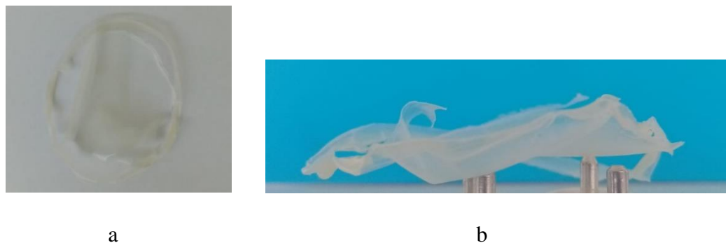
Figure 32. Top (a) and side (b) view of M1.b that was cast at an airflow rate of 40 L/s at 35 °C
