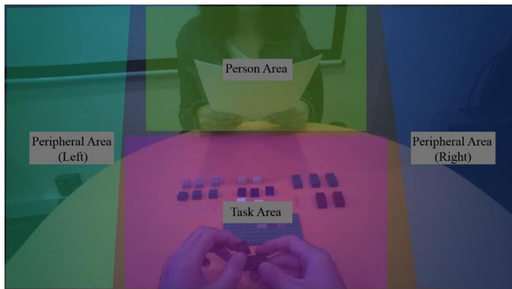
Figure 4. The setup for the dynamic AOI regions is displayed from the participant's field of view: Person Area (Facilitator), Task Area, Peripheral Area (Left), Peripheral Area (Right)
