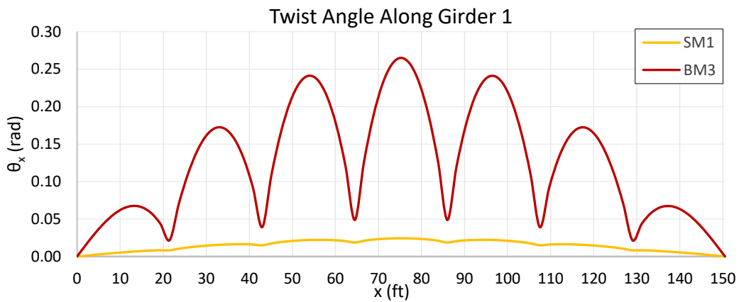
Figure 4-27 Twist angle along Girder 1 for models SM1 and BM3.
