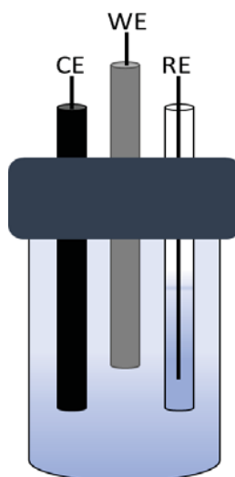
Figure 2.2. Schematic representation of the three-electrode system used for electrochemical measurements
