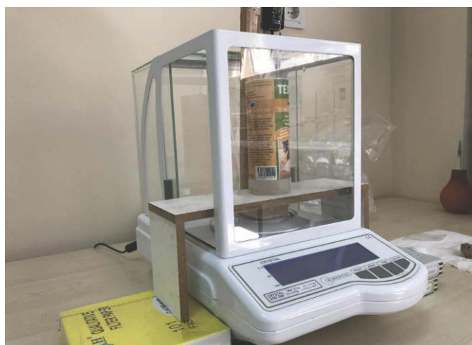
Figure 3.6. The Gibertini Crystal 200 SMI magnetic compensation analytical balance used in this study
