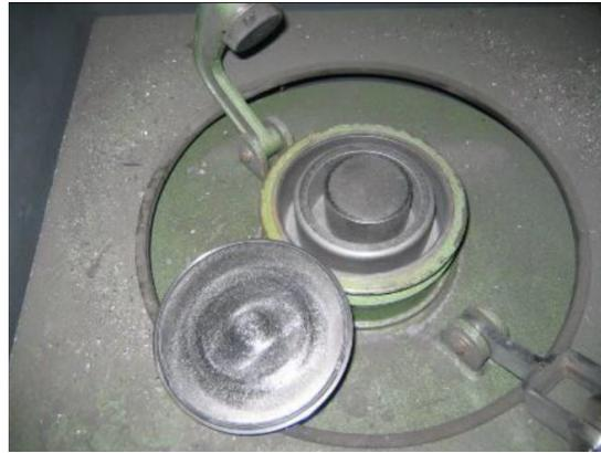
Figure 3.4: Ring mill grinder at Mineral Processing Laboratory METU
