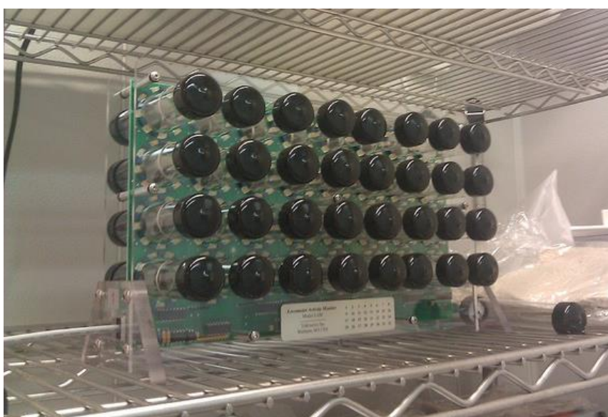
Figure 2.4. One of the activity monitors used in the experiments. The activity monitor has 32 cells and each cell can take 15ml (dimensions: 17 mm O.D., 120 mm length) falcon tube.
