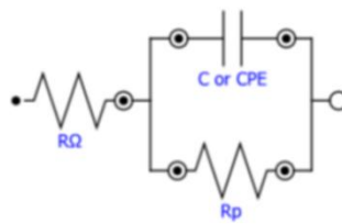
Figure 2.7. Simplified Randle's model as an equivalent circuit. R_{\Omega} : electrolyte resistance, R_p : polarization resistance, C/CPE: Capacitance/Constant phase element.
