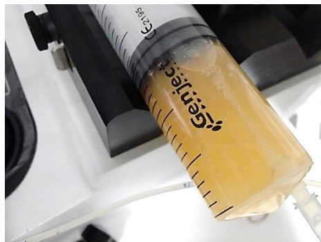
Figure 5.1. Bubbles formed inside analyte supply syringe.
