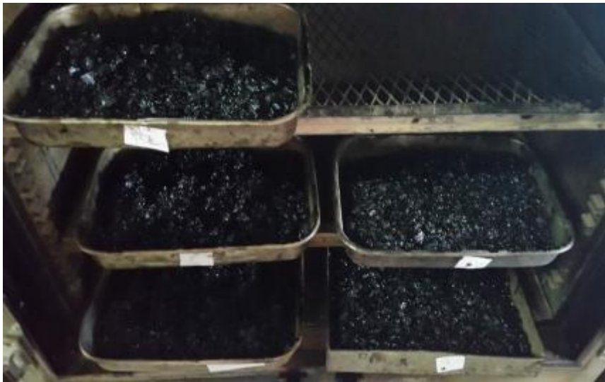
Figure 3.35. Loose HMA conditioned samples in the oven at compaction temperature
