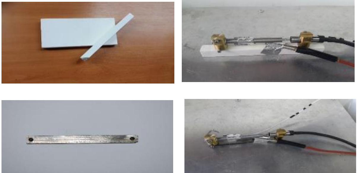
Figure 3.7. Test setup for calibration of LVDT and steel rod using ceramic and steel beam
