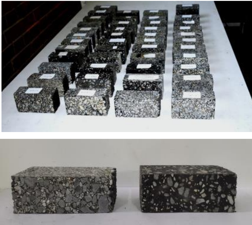
Figure 3.10. a) Prepared beam specimens for thermal coefficient measurement, b) Beam specimens before and after aging according to (AASHTO R30 2006)
