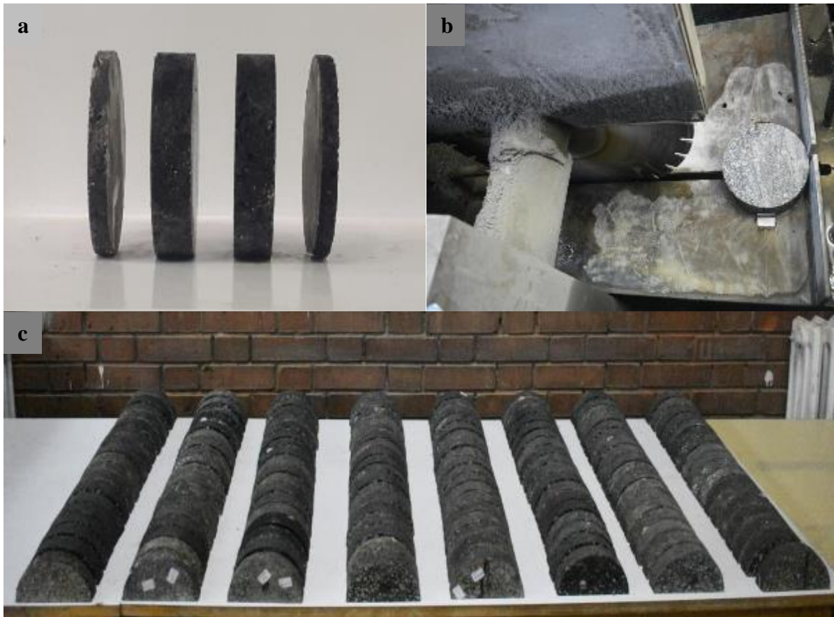
Figure 3.24. a) Sliced SGC specimen 35mm from center, b) cutting cylinder sample to obtain semicircular specimen, c) cut semicircular samples
