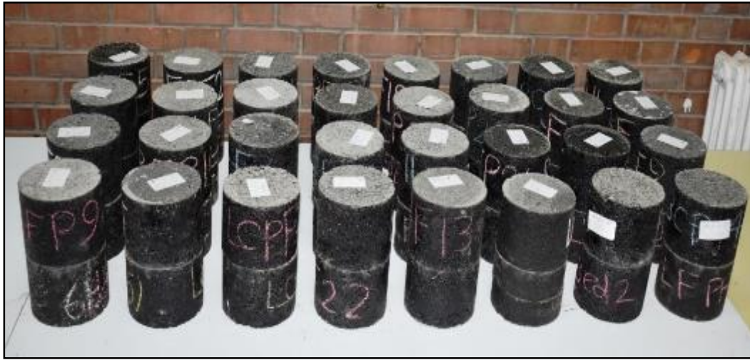
Figure 3.37. Compacted mix design samples according to the Superpave method
