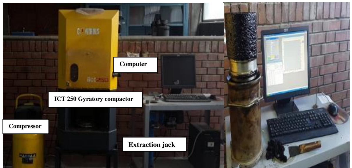
Figure 3.36. Sample compaction by gyratory compactor for Superpave design method (AASHTO T 312 2019)
