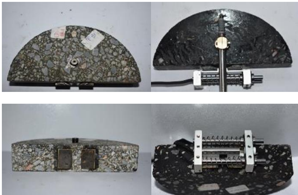
Figure 3.26. Attachment of gauges and LVDT to measure strains from CMOD and LLD
