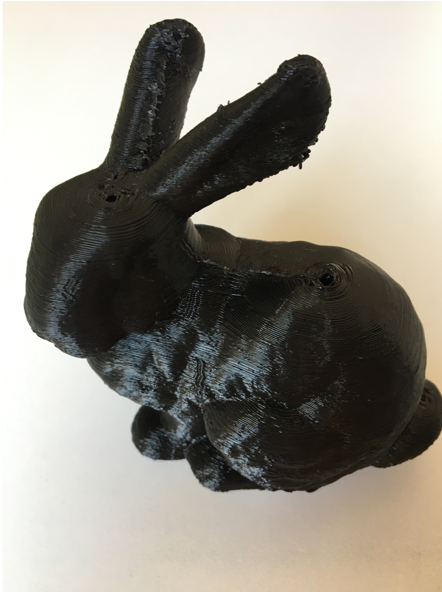
Figure 4.28: Bunny after the excessive material caused by insufficient fast travel feedrate is removed.
