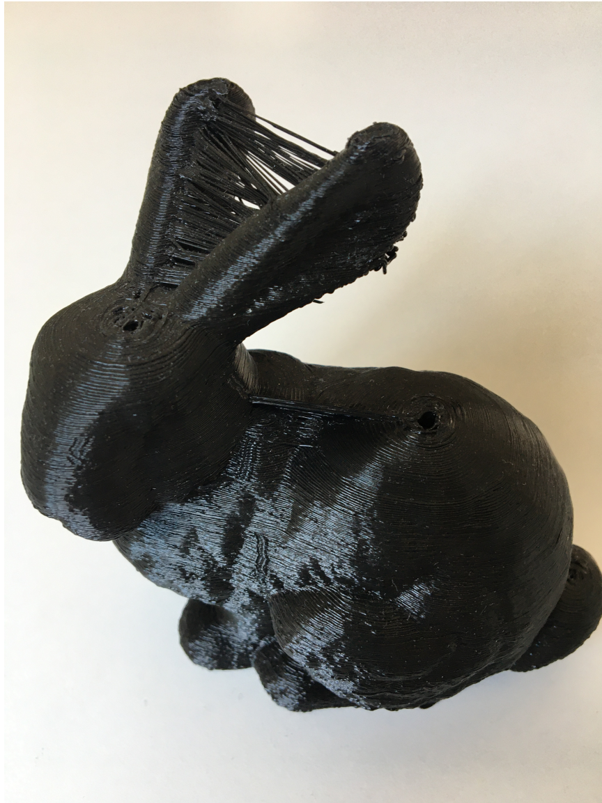
Figure 4.27: When feedrate of the printer head is not high enough in G0 motion, fast travels do result in solid lines.
