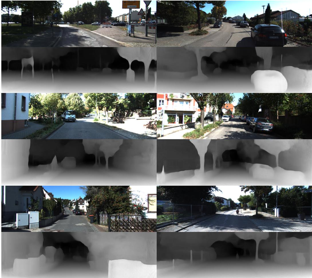
Figure 4.5: Some images and their depth estimation results, when Monodepth2 is trained with its default settings.
