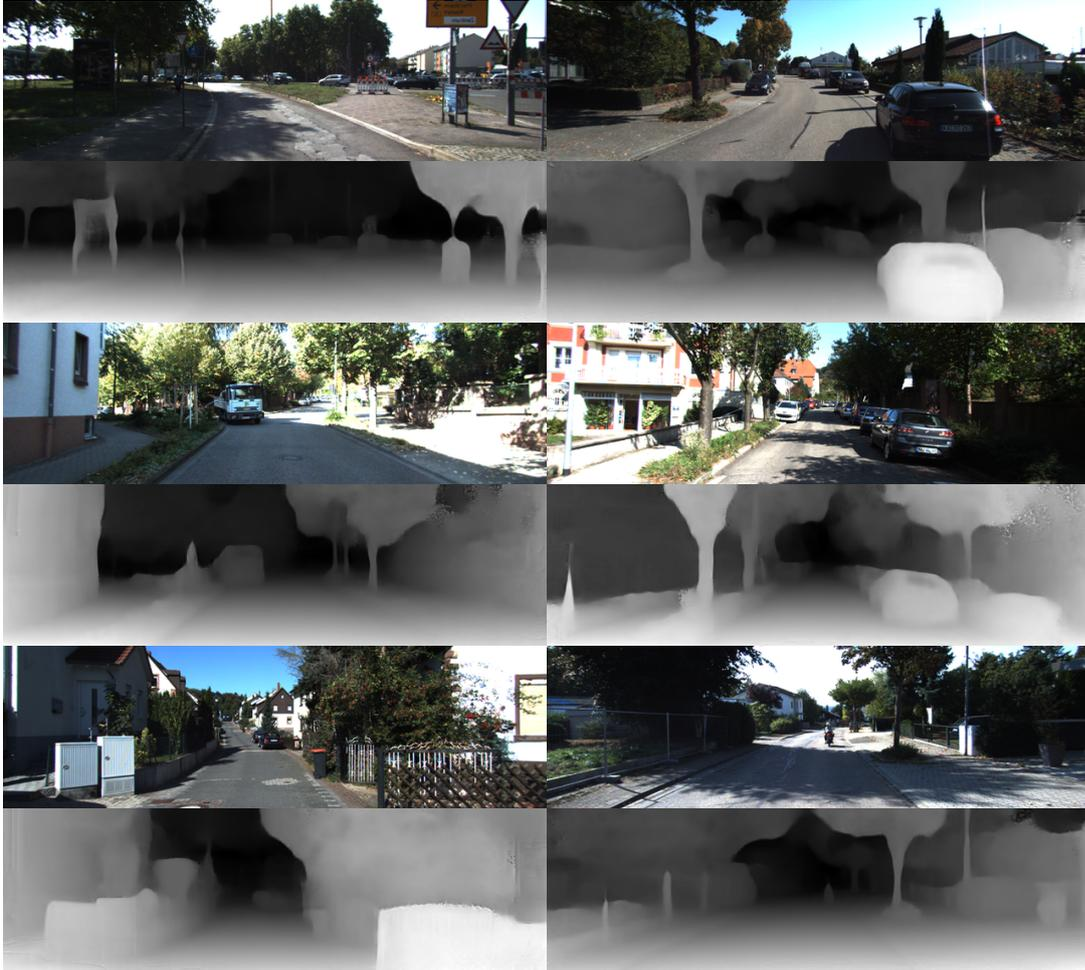
Figure 4.7: Some images and their depth estimation when Monodepth2 is trained with frames  $I_{\pm 7}$  as extra frames.
