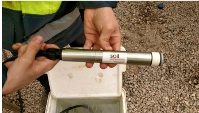
Figure 4.7. Vibrating wire piezometers installed in small diameter drill holes
