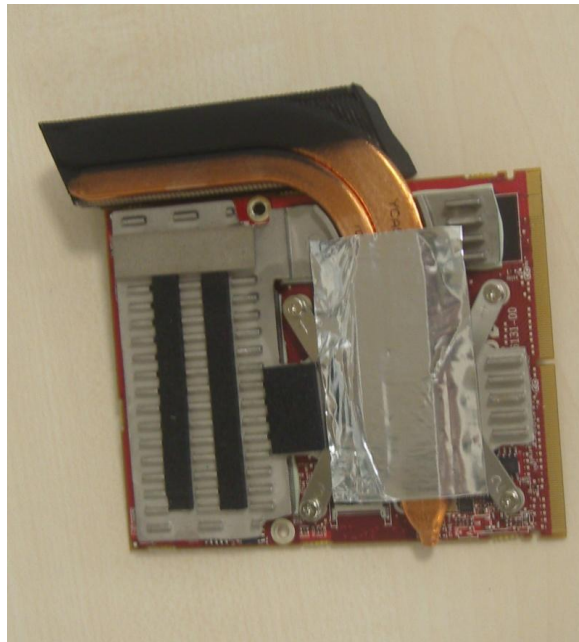
Figure 5.4 ATI Mobility Radeon HD 5870 model graphics card
