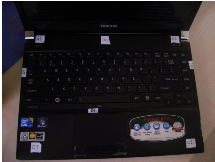
Figure 4.6 Toshiba external measurement points (top layer)
