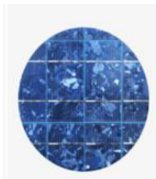
Figure 13: View of a polycrystalline PV panel (Verma & Singhal, 2015)
