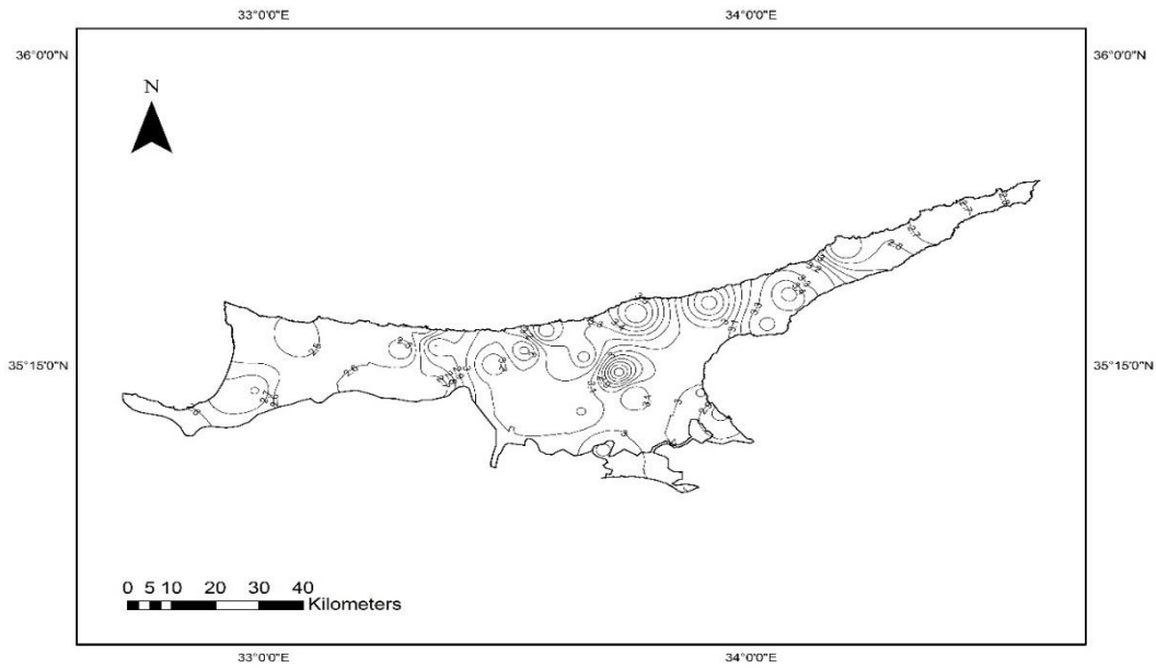
Figure 5.31 Isoseverity map of North Cyprus for 2-months drought duration and 10 year return period using SPI
