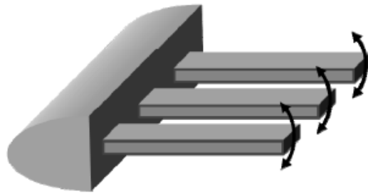
Figure 5.1. Schematic diagram of cantilevers beside each other [35].
