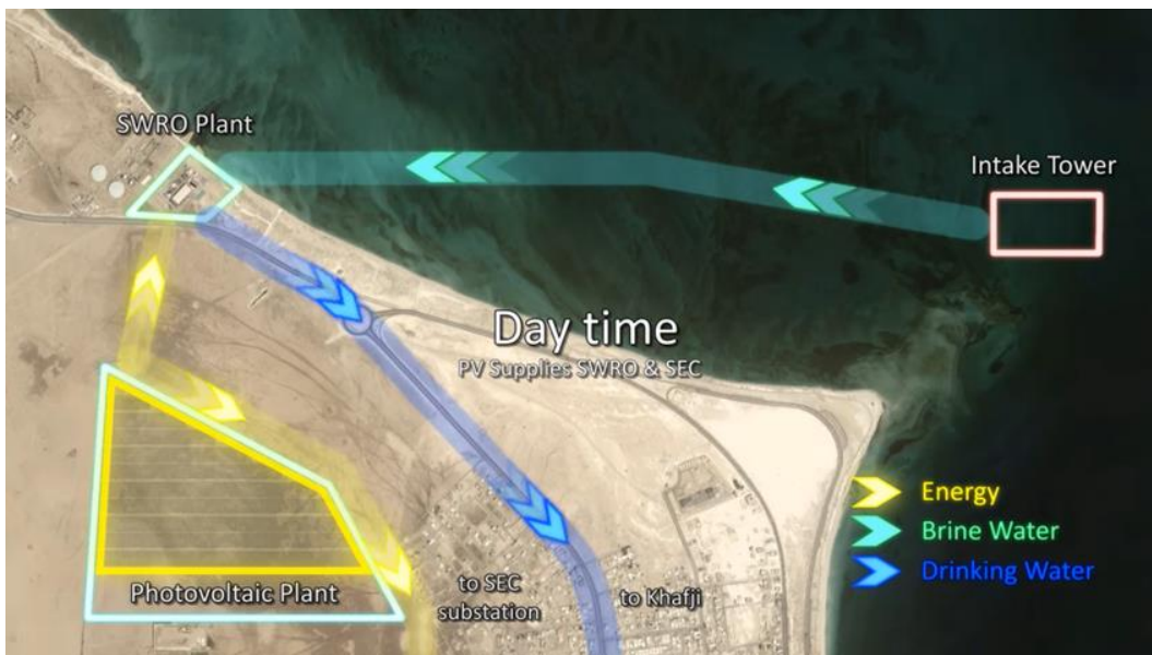
Figure 3-13 Al Khafji Solar Saline Water Reverse Osmosis day time working scheme
