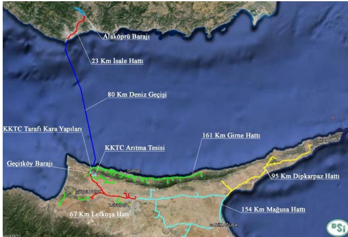
Figure 2-6 Northern Cyprus Water Supply project route, distances and planned pipeline infrastructure [44].
