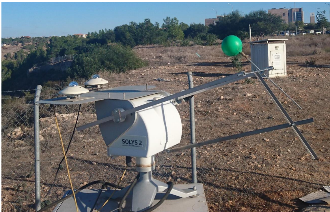
Figure 20. METU NCC solar station with manufactured shading ball.
