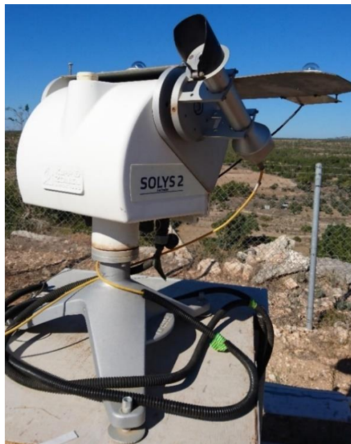
Figure 18. METU NCC solar station without shading ball.
