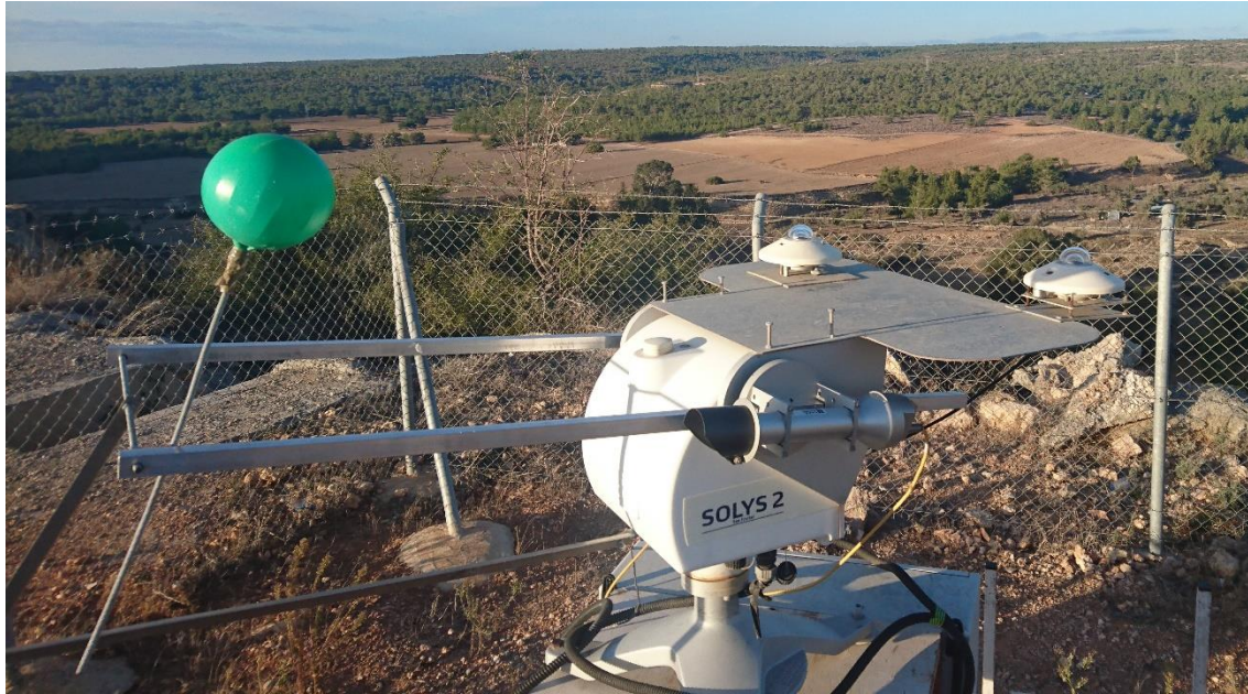
Figure 19. METU NCC solar station with manufactured shading ball.
