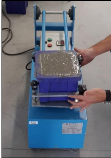
Figure 3.11. Vibrators providing compaction to fully filled concrete mold.
