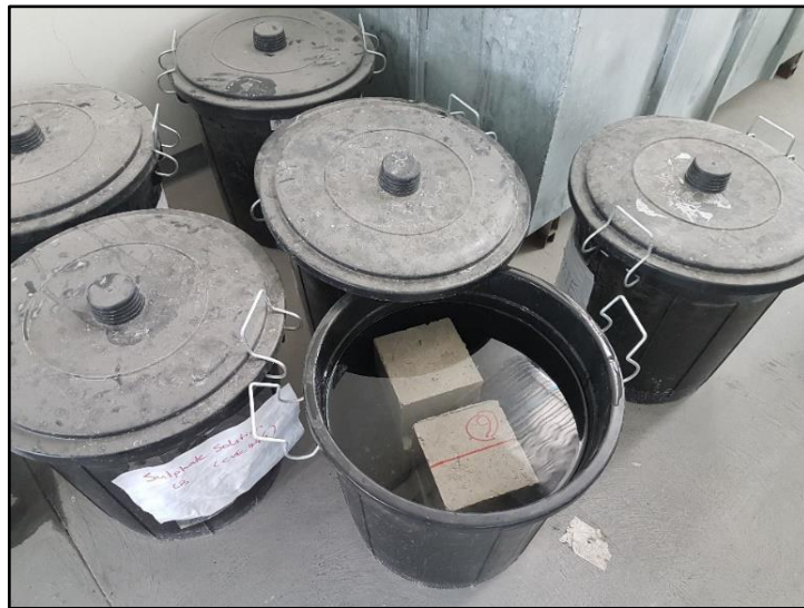
Figure 3.17. External sulfate attack curing condition.
