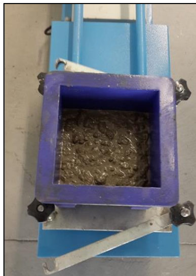
Figure 3.10. Vibrators providing compaction to half-filled concrete mold.
