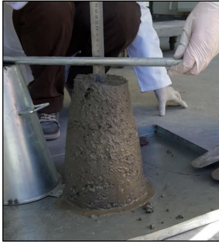
Figure 3.9. Slump measurement taken on fresh concrete.
