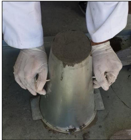
Figure 3.14. Determination of slump.
