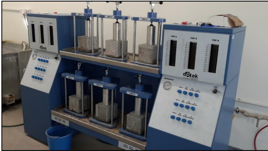
Figure 3.16. Water permeability testing equipment.
