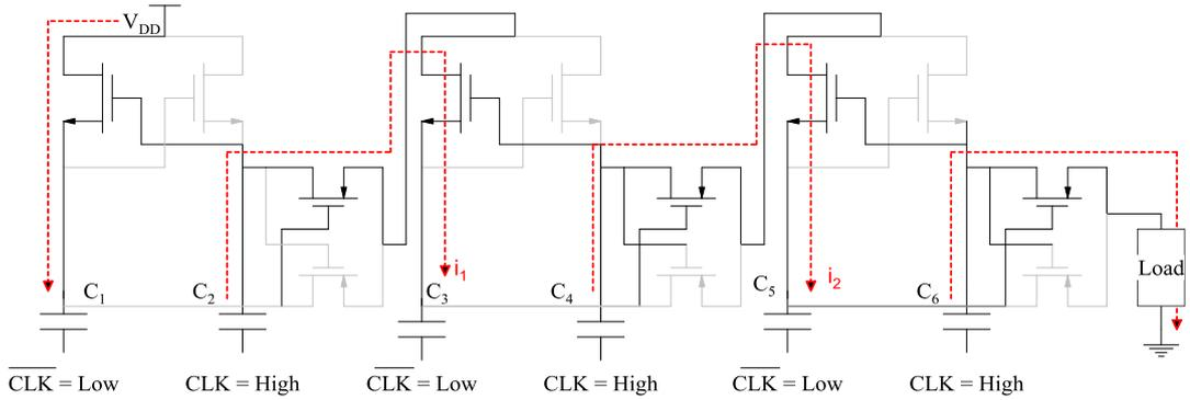
Figure 3.11. ON and OFF paths in a 3 stage charge pump at the instant that  $CLK_n = high$  and  $CLK_{n+1} = low$ .
