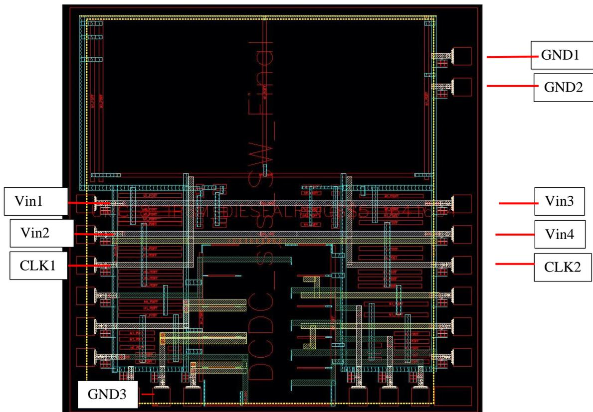
Figure 6.15. Location of the pins used for resistance measurement on the layout.
