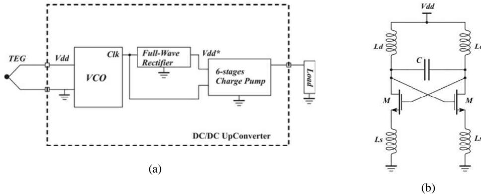
Figure 3.4. (a) DC-DC converter topology using LC-tank oscillators first proposed in [47], (b) VCO Circuit.
