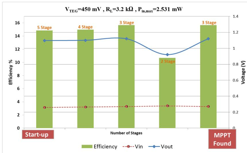
Figure 6.27. Measurement results for the autonomous system with  $V_{TEG}=450$  mV and  $3.2$  k $\Omega$  load.
