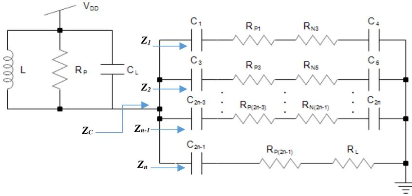
Figure 3.12. The half circuit model proposed for the model based design optimization to deliver maximum power [49].
