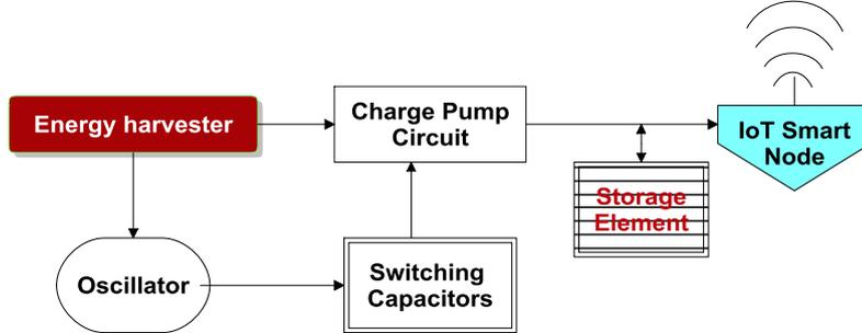
Figure 3.1. The block diagram of a charge pump based DC-DC converter for energy harvesting applications.
