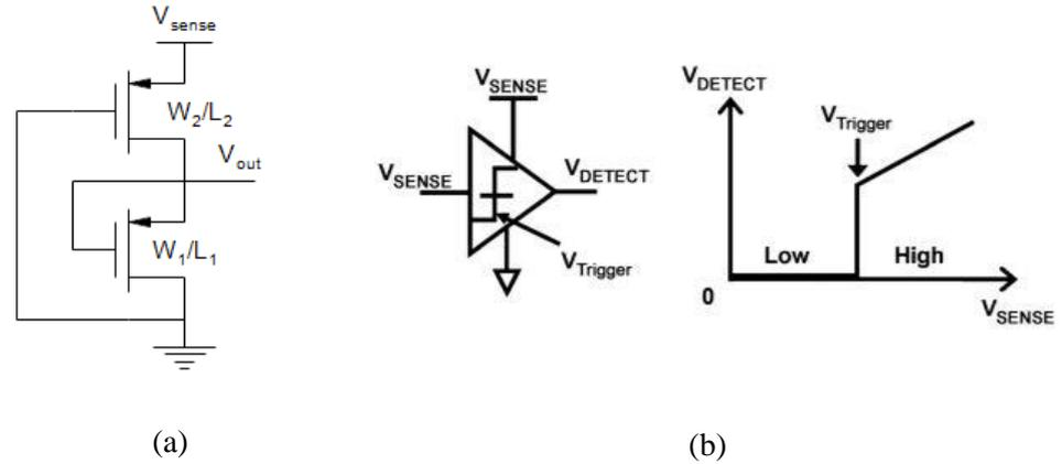
Figure 4.15. (a) The voltage level detector circuit, (b) Input-output characteristic [100].
