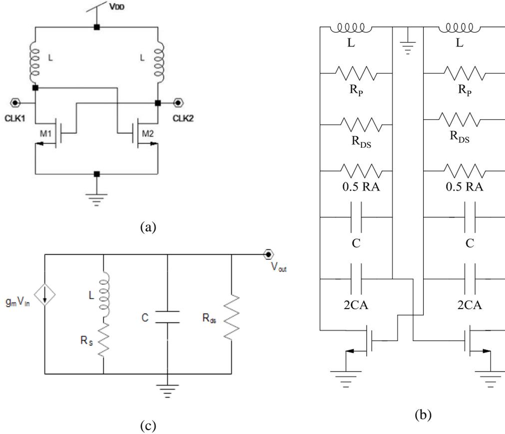
Figure 3.9. (a) The oscillator circuit topology with minimum number of elements, (b) circuit model of the LC-tank and the cross coupled NMOS transistors that create the negative resistance necessary to sustain the oscillation, and (c) simplified model of the oscillator [49].
