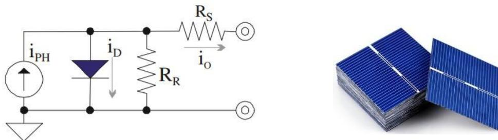
Figure 2.2. (a) Typical one diode PV cell model [11]. (b) Sample miniature PV cells for micro-scale solar energy harvesting 22 mm × 17 mm TSPV, 1 mW at MPP.
