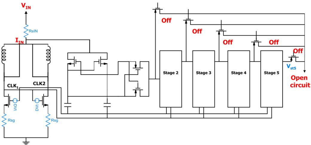
Figure 6.12. The proposed model for the DC analysis of fabricated NMOS mismatch with the simulated results.
