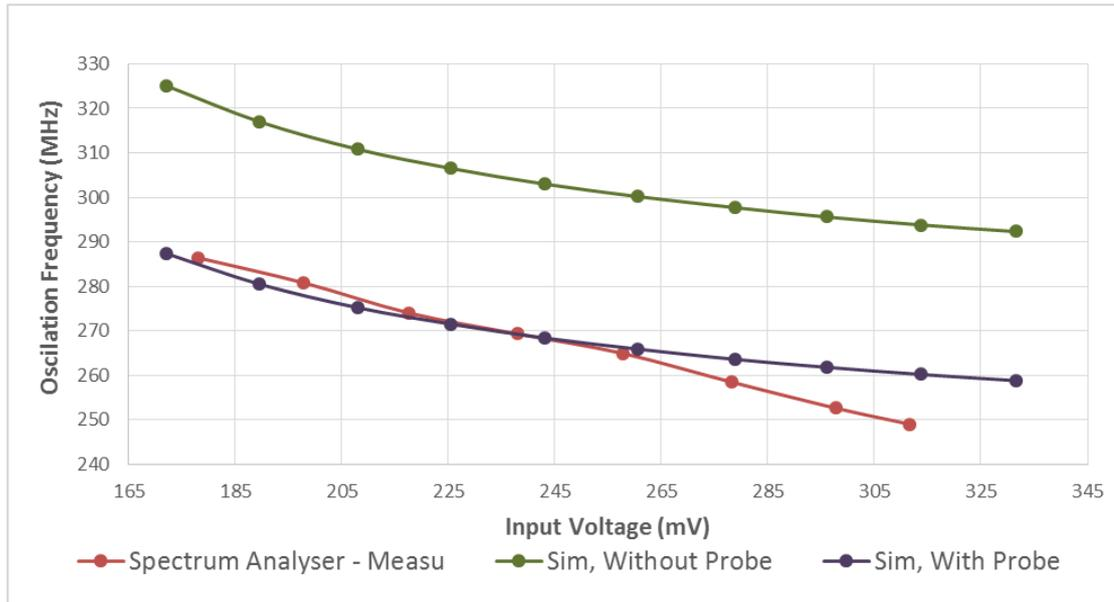
Figure 6.18. Comparison of oscillation frequency of the modified model and the measurement results.
