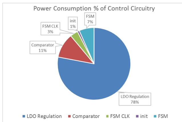
Figure 5.6: The histogram of the power consumption of different blocks of the fully autonomous system.
