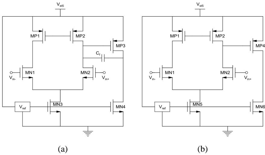
Figure 4.16. (a) Op-Amp circuit (b) Comparator circuit
