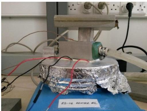
Figure 6.29. The TEG set-up to provide the necessary temperature difference.
