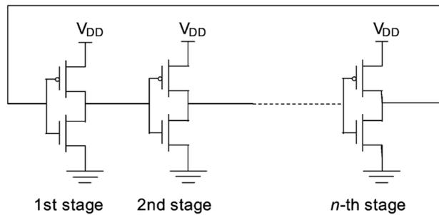
Figure 3.3. Topology of the ring oscillator circuit (odd  $n$ ).
