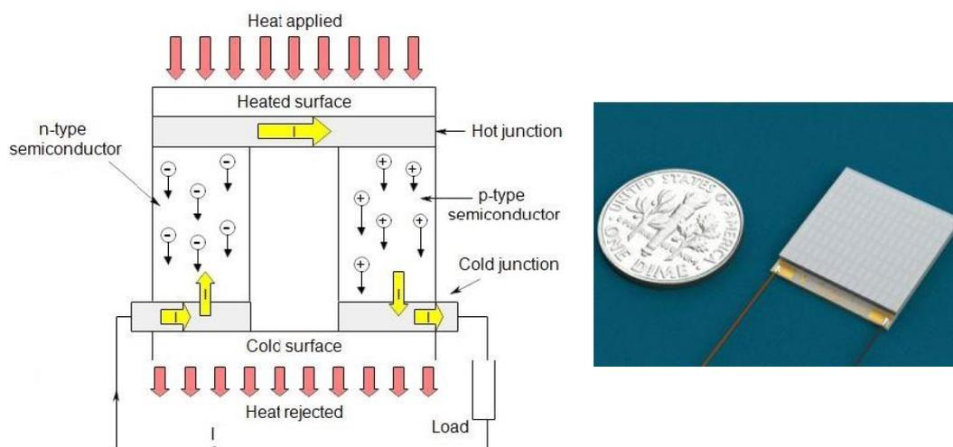
Figure 2.4. (a) Thermoelectric generator based on the seebeck effect (b) tiny TEG for micro-scale energy harvesting, 16 mm × 16 mm TEG, 0.2 mW at MPP [24].
