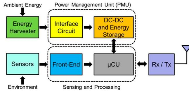
Figure 1.2. Block diagram of an IoT smart node [7].
