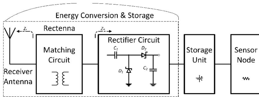
Figure 2.11. RF energy harvesting circuit components [22].
