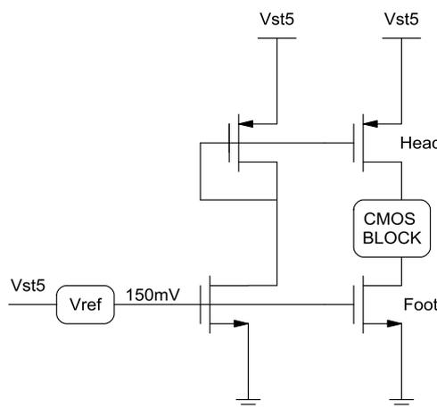
Figure 4.7. Pushing the CMOS block to operate in subthreshold region using Foot and Head MOSFETs.
