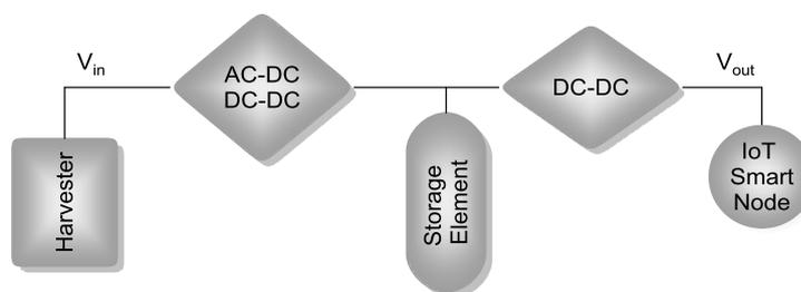
Figure 1.3. Harvesting microsystem composed of harvester and interface circuit [11].
