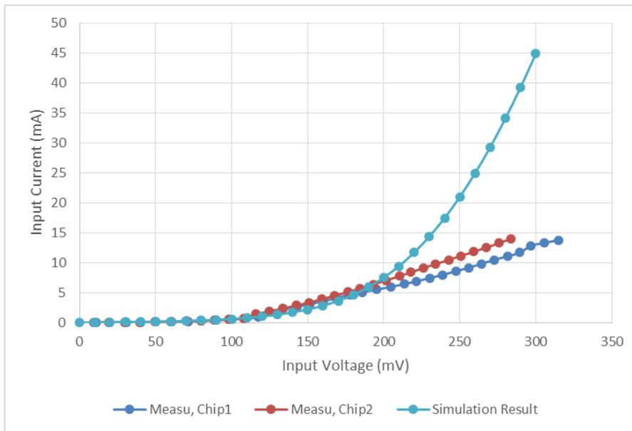
Figure 6.11. I-V curve of the circuit shown in fig. 5. 10.
