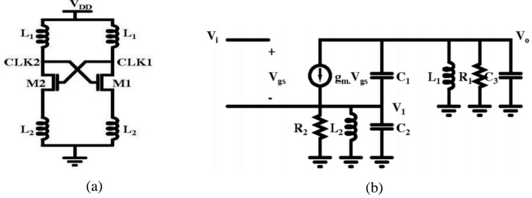
Figure 3.8. (a) The proposed LC-tank topology and (b) the corresponding half circuit model for optimization [46].
