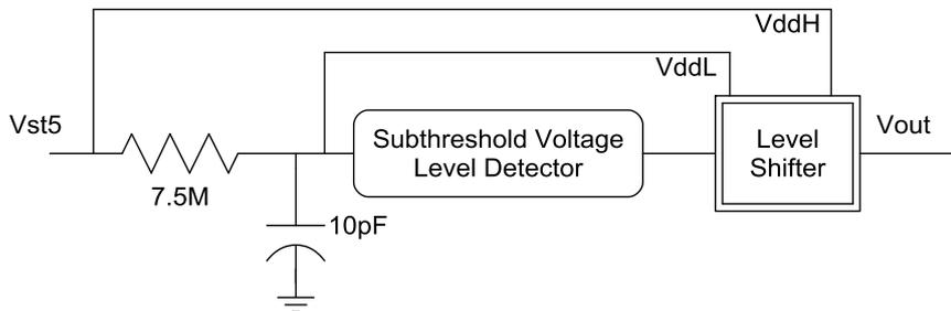
Figure 4.14. Initialization circuit that generates the required pulse for initializing the FSM.
