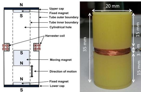
Figure 2.9. Electromagnetic energy harvester [21].
