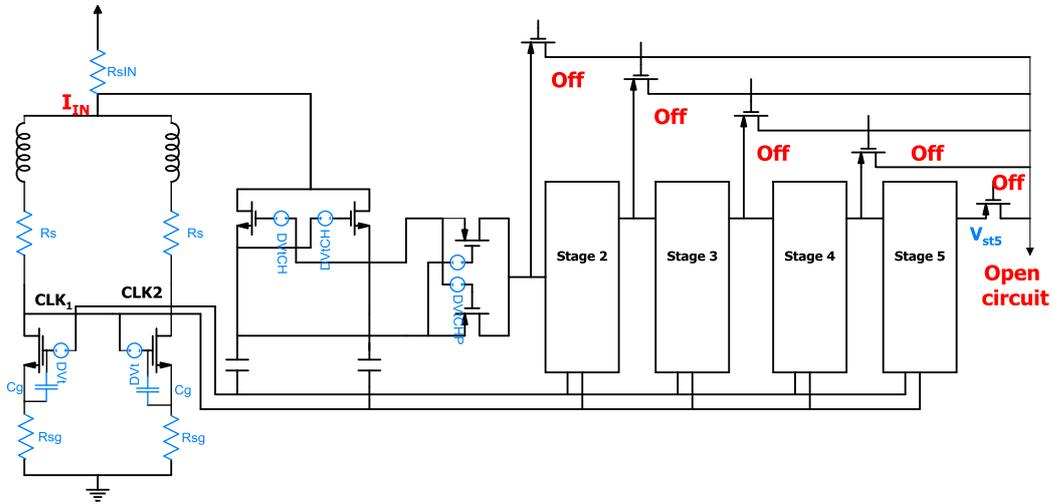
Figure 6.24. The final model elements that describe the discrepancy between the post layout simulation and the fabricated chip.
