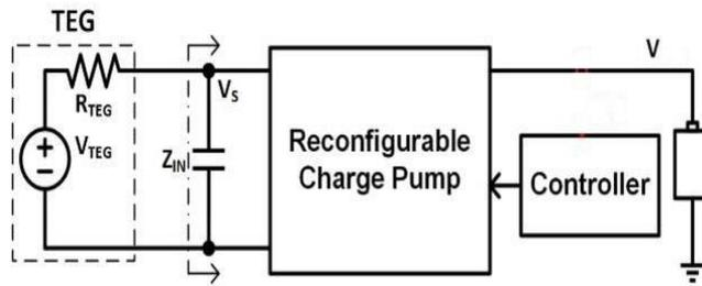
Figure 3.14. Schematic diagram of charge pump based DC-DC converters with maximum power point tracking capability.
