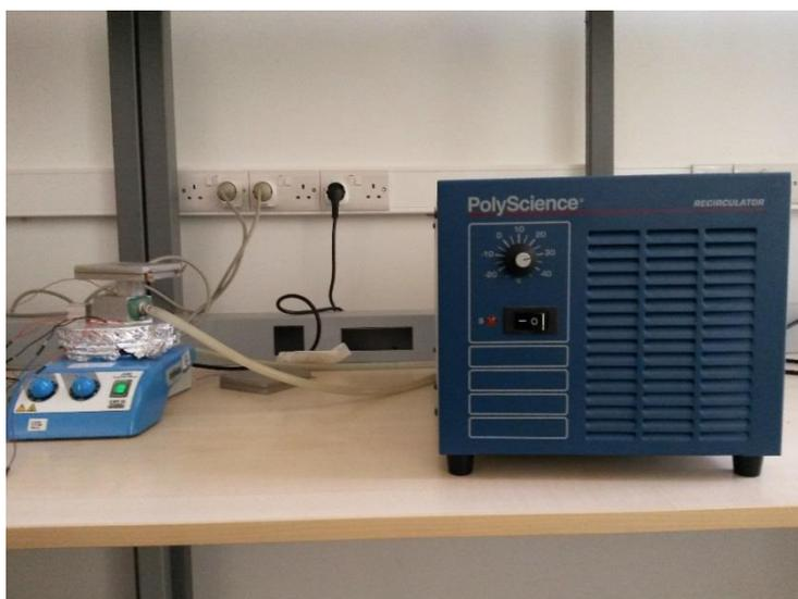
Figure 6.30. The cooler and heaters used for TEG cold and hot palates.
