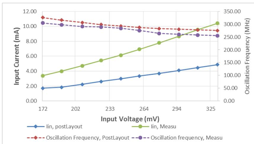
Figure 6.9. Oscillation frequency and input current for post-layout simulation versus measurements.
