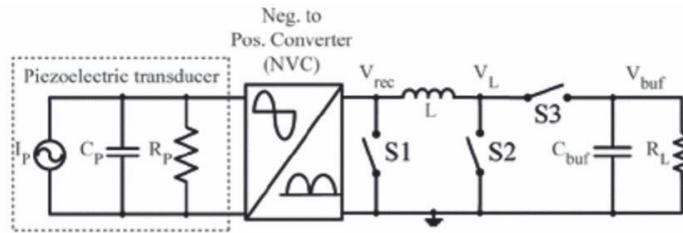
Figure 2.8. Schematic of a SECE interface for piezoelectric energy harvesters.
