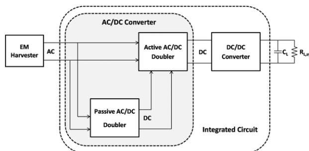
Figure 2.10. The integrated interface block diagram of the electromagnetic energy harvester [21].
