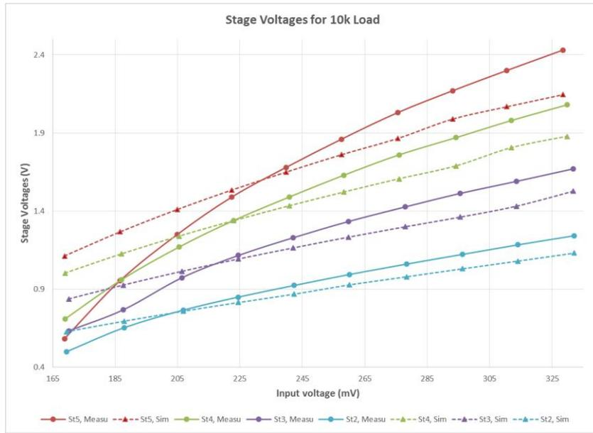
Figure 6.22. Comparison of the output voltage of the stages between simulation of the modified model and measurement results for 10 kΩ load.
