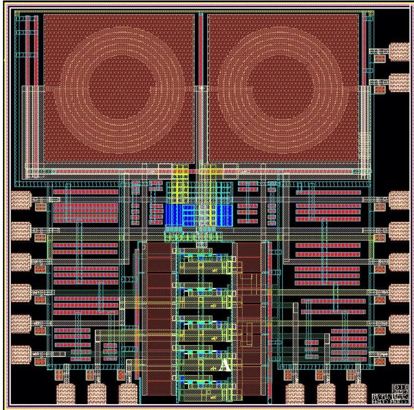
Figure 6.2. Chip layout photo with PAD connections.
