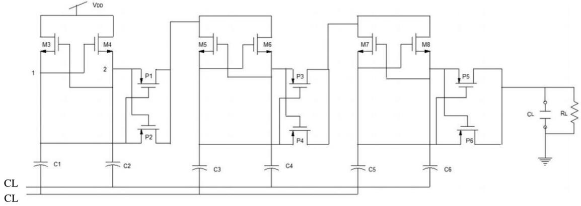
Figure 3.10. The charge pump circuit topology for a three stage charge pump used in [49].
