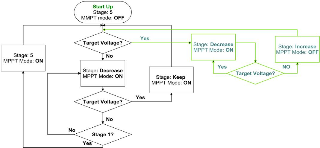
Figure 4.4. The proposed novel MPPT algorithm for charge pump based DC-DC converters with LC-tank oscillator.
