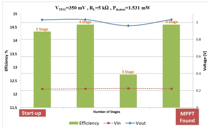
Figure 6.26. Measurement results for the autonomous system with  $V_{TEG}=350 \text{ mV}$  and  $5 \text{ k}\Omega$  load.
