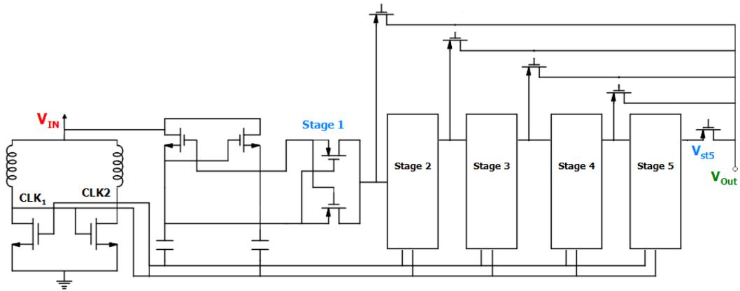
Figure 4.2. The proposed topology to create a charge pump with variable number of stages.
