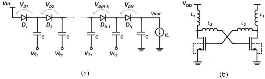
Figure 3.5. (a) The DC-DC converter topology using initially proposed LC-tank oscillators, (b) VCO circuit [55].
