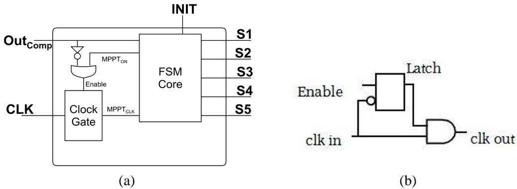
Figure 4.6. (a) Block diagram of the MPPT circuit (b) Clock gating block.
