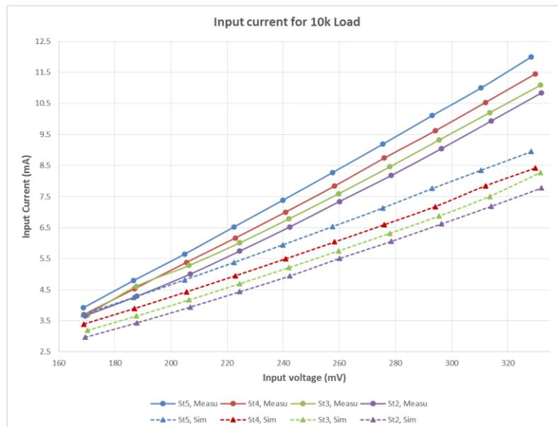
Figure 6.23. Comparison of the input current between simulation of the modified model and measurement results for loads of 10kΩ.
