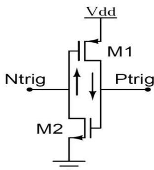
Figure 4.10. A conventional CMOS Thyristor block.
