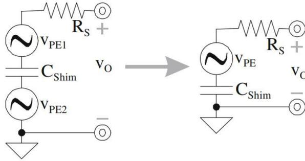
Figure 2.7. Circuit equivalent model for the piezo electric harvester [11].
