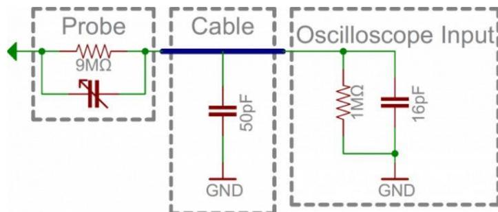
Figure 6.19. The oscilloscope probe model [104].
