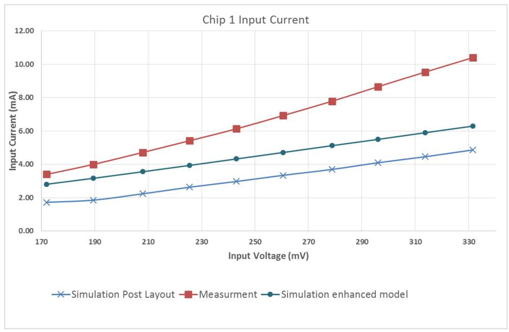
Figure 6.17. The comparison of the input current with respect to the input voltage change against the modified model no-load scenario.
