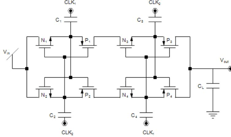
Figure 3.2. Dual-phase charge transfer cross-connected charge pump [37].
