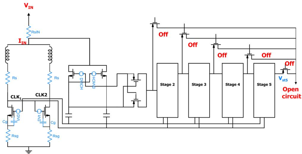
Figure 6.14. The modified model that identifies the parasitic elements that describe measurement data and post layout simulation discrepancy.
