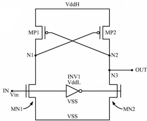
Figure 4.13. Voltage level shifter.
