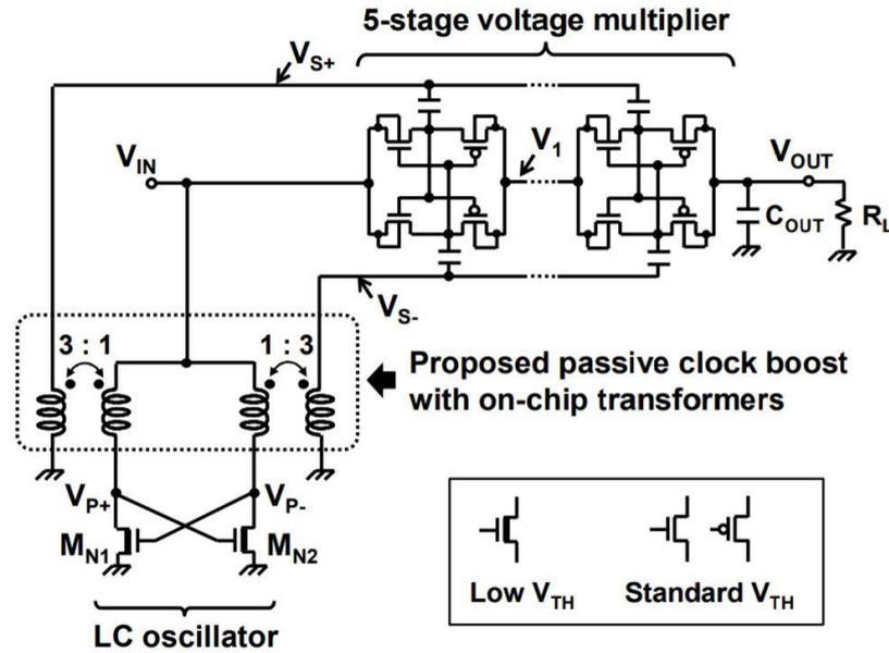
Figure 3.6. The circuit schematic of the fully integrated DC-DC converter proposed in [56].
