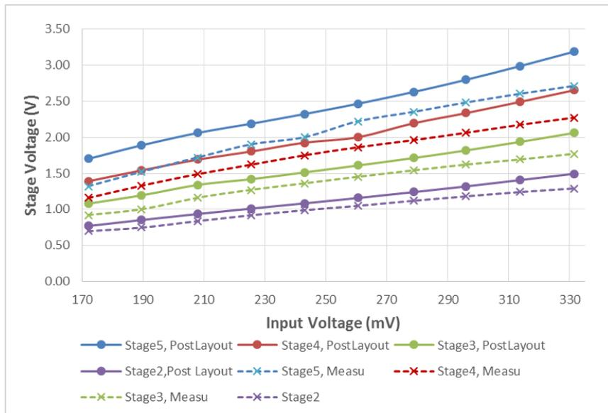
Figure 6.8. Stage voltages for post-layout simulations versus measurements.
