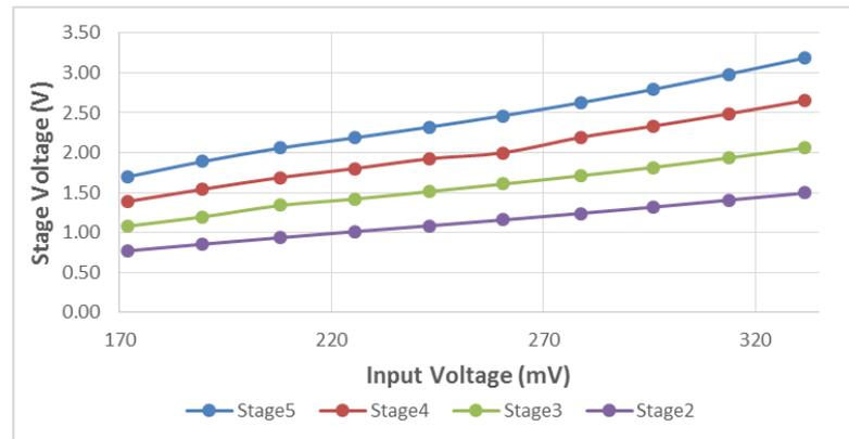
Figure 6.6. Post layout simulation results for output voltage from different stages with respect to varying input voltage and no load condition.
