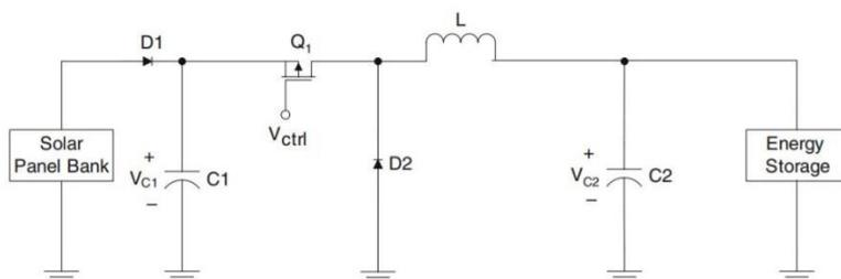
Figure 2.3. Block diagram of an interface circuit for solar energy harvesting [13].
