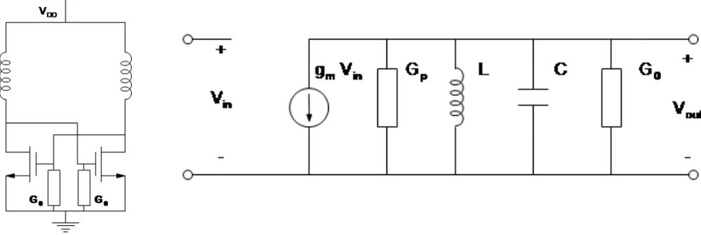
Figure 4.1. LC-tank small signal model with Charge pump modeled as the load. [71]
