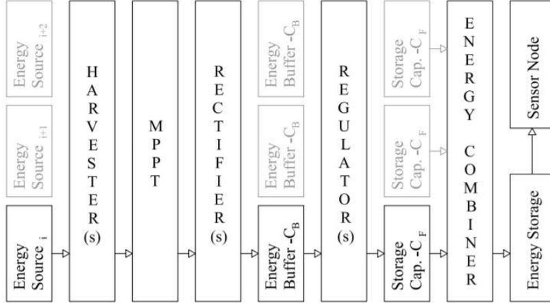
Figure 2.12. Block diagram of a hybrid energy harvesting system when only a single source is present [24].
