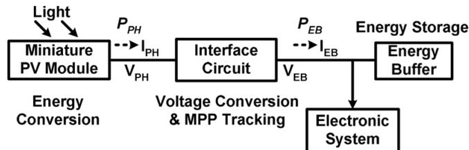
Figure 2.1. The building blocks of a smart node based on solar energy harvesting [12].
