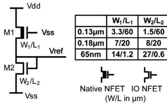
Figure 4.9. Ultra-low power voltage reference proposed in [89].
