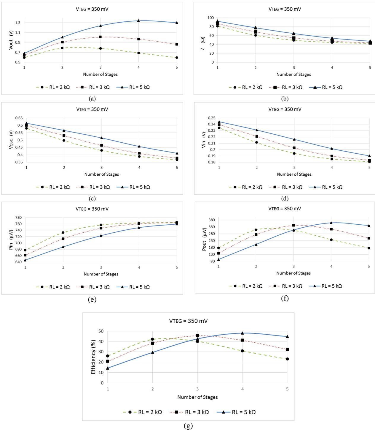
Figure 5.1. Simulation results of the behavior of the DC-DC converter for varying load and fixed Source voltage. (a) For each load there is one stage which provides maximum output voltage. (b) Input impedance of the system decreases as number of stages increases. (c) As number of stages increases charge pump loading reduces the oscillation amplitude. (d) For a fixed VTEG,  $V_{in}$  has inverse relation with number of stages. (e) Input power is maximum in
