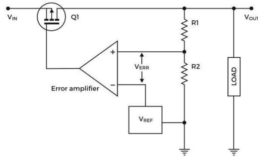
Figure 3.15. The block diagram of a typical low-dropout regulator.
