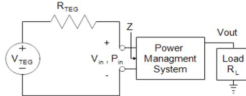
Figure 4.3. The block diagram of the energy harvesting system with respect to the first order TEG model.
