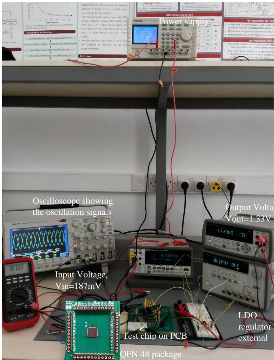
Figure 6.5 . Experimental setup for the system validation.
