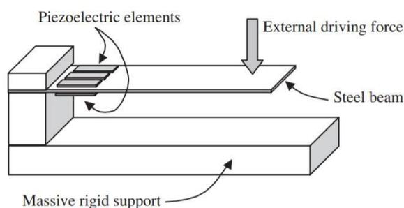
Figure 2.6. Schematic of the typical setup for piezoelectric energy harvesting [19].
