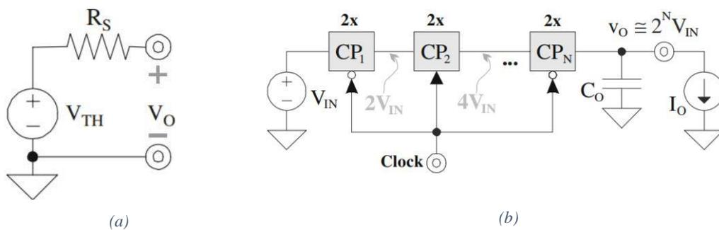
Figure 2.5. (a) TEG model, (b) A typical Interface circuit for voltage boost up based on charge pump [11].
