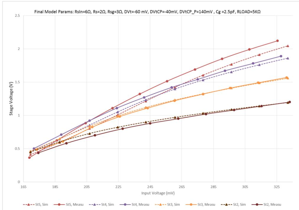
Figure 6.25. Stage output voltages match between the measurement data and the final model.
