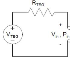
Figure 3.13. First order model widely accepted for thermoelectric generators.
