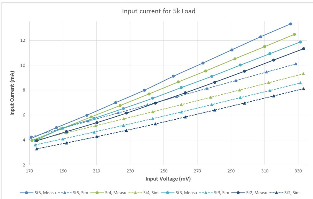
Figure 6.21. Comparison of the input current between simulation of the modified model and measurement results for 5 kΩ load.
