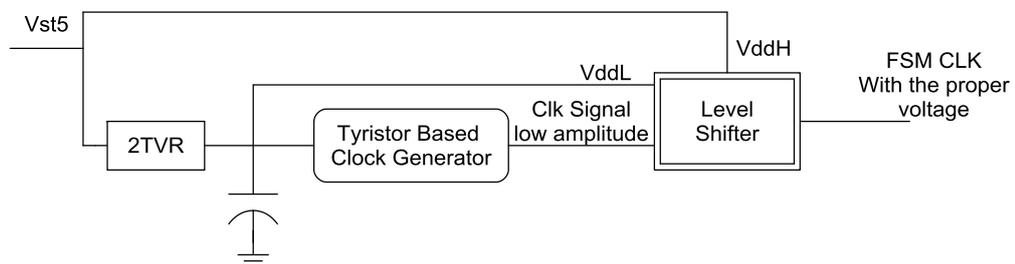
Figure 4.12. The proposed circuit topology for ultra-low power FSM clock generator.
