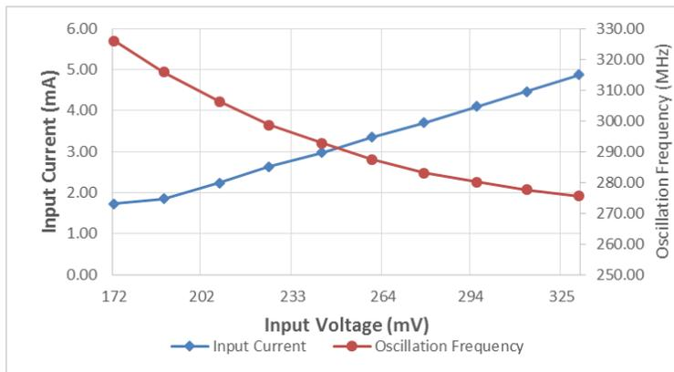
Figure 6.7. Post layout Simulation results for the input current and oscillation frequency with respect to varying input voltage and no load condition.
