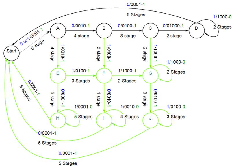
Figure 4.5. The state diagram of the proposed MPPT algorithm.
