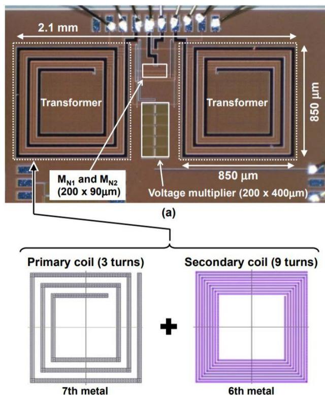
Figure 3.7. The chip micrograph of the circuit proposed in [56] and implemented in 65 nm technology.
