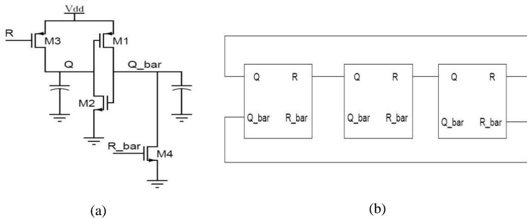
Figure 4.11. (a) A typical delay element created by the CMOS thyristor gate, (b) block diagram of a three stage thyristor based ring oscillator [99].
