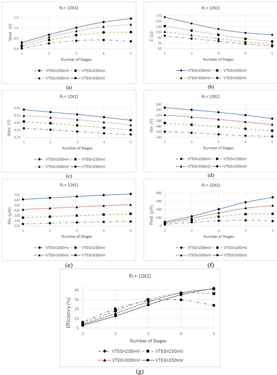
Figure 5.2. Simulation results for the proposed power management system behavior with a fixed load and varying  $V_{TEG}$ . (a) For different  $V_{TEG}$  there is one stage which provides maximum output voltage. (b) Input impedance of the system decreases as the number of stages increases.
