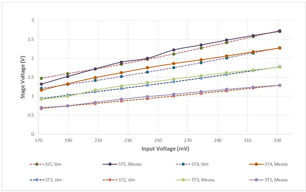
Figure 6.16. The comparison of the output voltage of the stages with respect to the input voltage change against the modified model no-load scenario.
