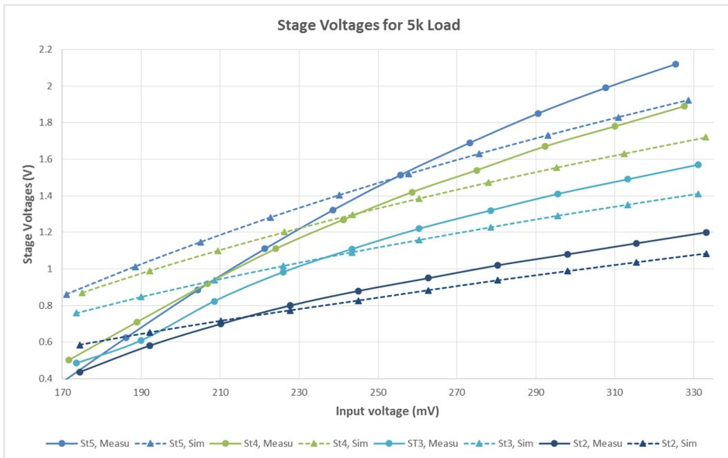
Figure 6.20. Comparison of the output voltage of the stages between simulation of the modified model and measurement results for 5 kΩ load.
