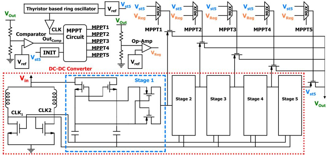
Figure 4.8. The schematic of the overall fully autonomous integrated power management system.
