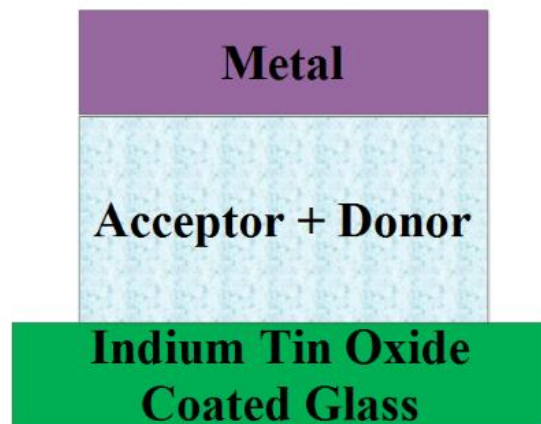
Figure 2.8. Bulk Heterojunction Solar Cell
