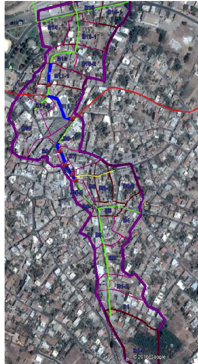
Figure 47. Junctions and conduits in Subcatchment B that face problem in 25 mm/h rainfall event.
