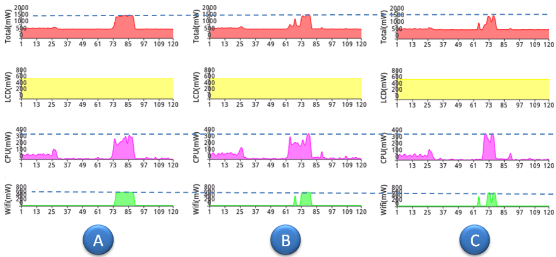
Figure B.3: Power Consumption While Browsing Aliexpress without Twes+(A), with Twes+ and without Resizing Feature (B), and with Twes+ and Resizing Feature (C)
