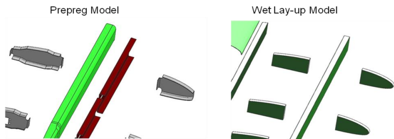
Figure 8: Comparison of the Spars and Ribs of Composite Wing Models, Close-up View
