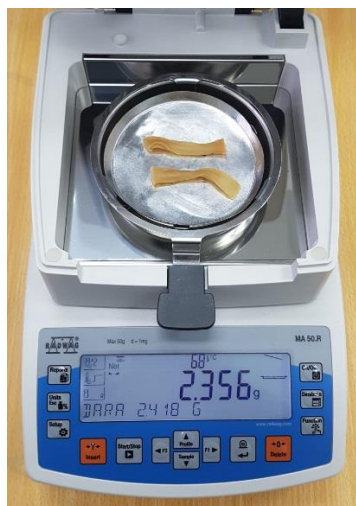
Figure 3. Dried thin layer samples in IR dryer
