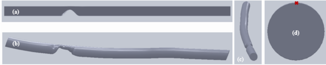
Figure 1: (a) Idealized model, (b, c) Realistic model, (d) location of the line on the vessel wall along which pressure is collected
