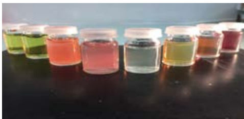
Figure 1: Different metal and semiconductor nanoparticles obtained using the proposed laser ablation methodology
