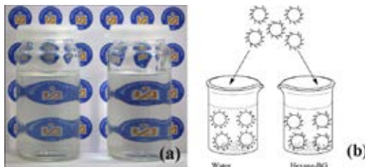
Figure 2: (a) Picture of 10% by weight of sample 4B in water (left) and hexane-BG (right). (b) Illustration of preparation of TiO 2 hydrosols in water and hexane-BG.
