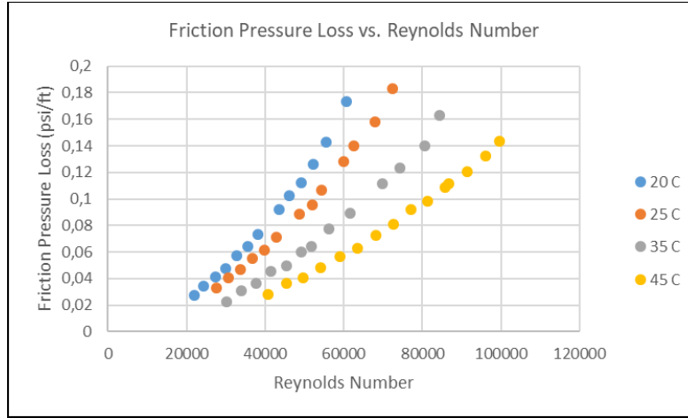
Figure 2: Friction Pressure Loss vs. Reynolds Number for Water
